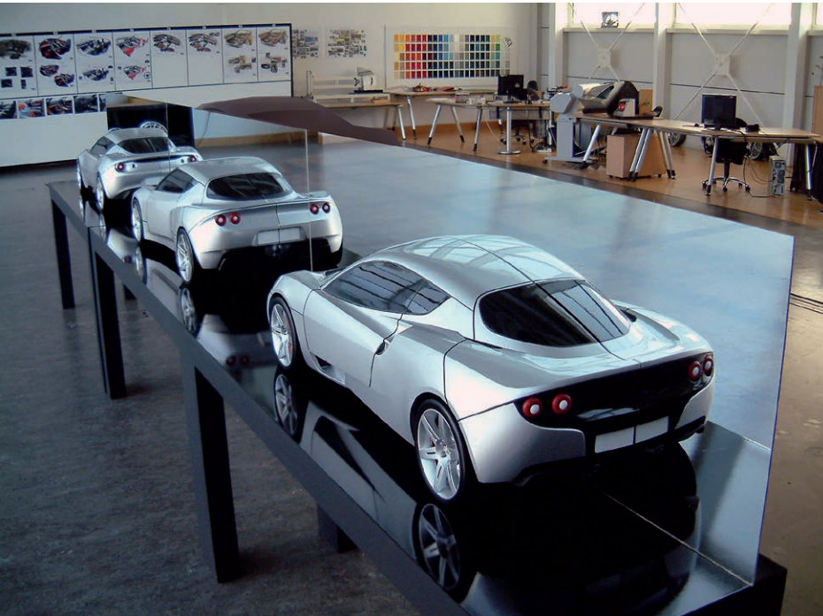
The clay models representing the final three possible iterations of the Evora, one of which got the nod. (Courtesy Lotus Cars)
