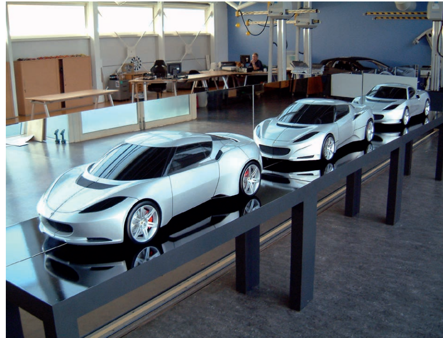
Mirror image: front-three-quarter view of the three finalists for the Evora design; certain features such as the front splitter would appear in subsequent production versions. (Courtesy Lotus Cars)
