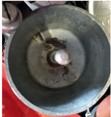
3-5: Corrosion in float chamber.
