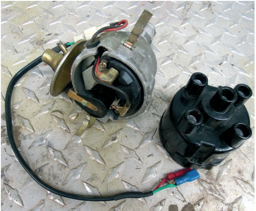
You can incorporate modern technology with electronic ignition, which is usefully immune to distributor shaft wear. Doesn't work for me; does work for most people.
