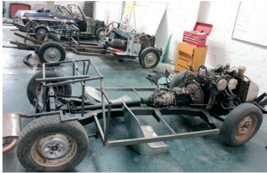
The Spitfire chassis in the foreground differs from the Herald chassis behind only in being 8in shorter and having no rear outriggers. The mechanicals are virtually interchangeable.
