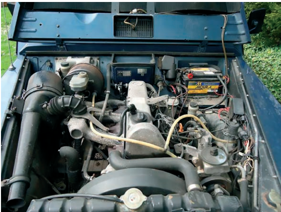
The M103 had early head gasket/oil leaks, usually from the area indicated above; revised head gaskets remedied this, however.
