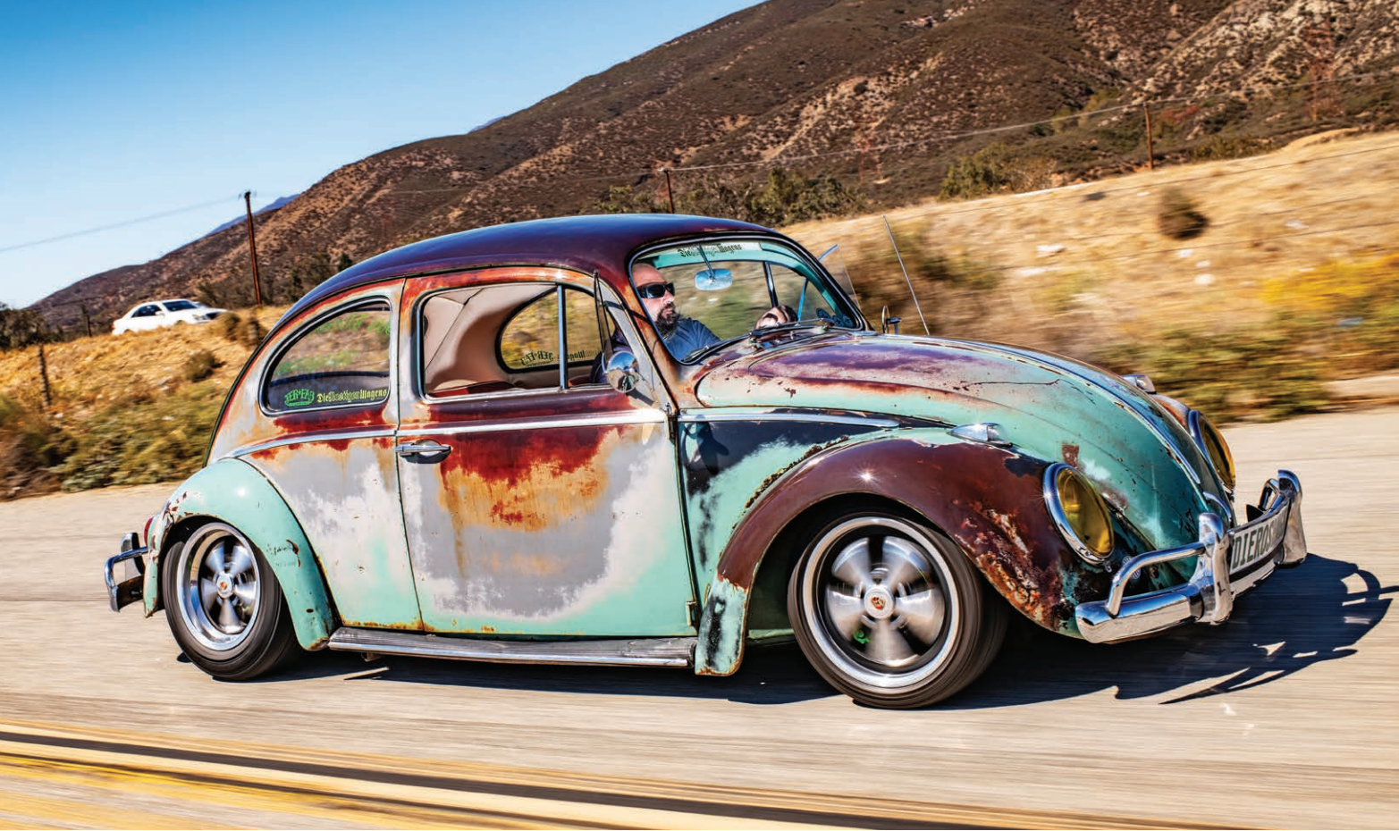
When attempting to convincingly blend paint onto a car like Nick Bevis' Turkis Bug, you'll need to match the paint to several different areas and carefully mask up large areas when adding paint. (Courtesy Andrew Thompson/AThompsonsPhoto)
