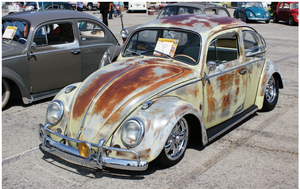
Volkswagen used different primer colours on different coloured cars, as well as two different coloured primer layers – matching both primer colours as well as the topcoat will result in a much better finish. (Courtesy @10ft_Doug)
