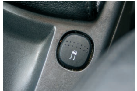
ST170 has TC or ESP button to disable the system.
