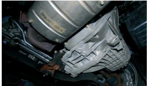
RS transmission incorporates limited-slip differential; check 'box for worn synchromesh.
