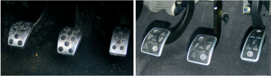
The rubber-studded aluminium ST170 pedals. RS's should have Sparco branding.
