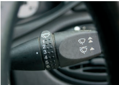
ST170 variable-speed wiper stalk may be retrofitted to RS.
