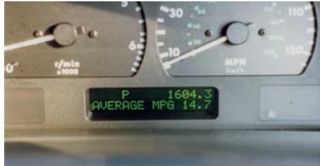
**The on-board computer of this early 4.6 HSE calculated the fuel consumption after around 200 miles of mixed driving. There was no reason to argue ...**
