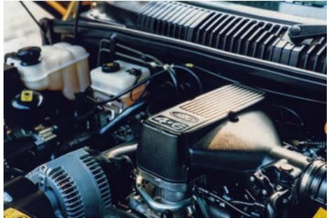
**The thirstiest engine of all is the 4.6-litre V8, seen here in an early model. The later ‘Thor’ engines had a different appearance, with a tubular manifold on top of the engine.**
