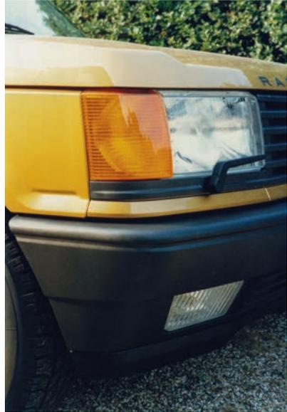
**The condition of the four corners gives a good clue to how well the vehicle has been looked after. Scrapes will be very noticeable on the later painted bumper aprons.**
