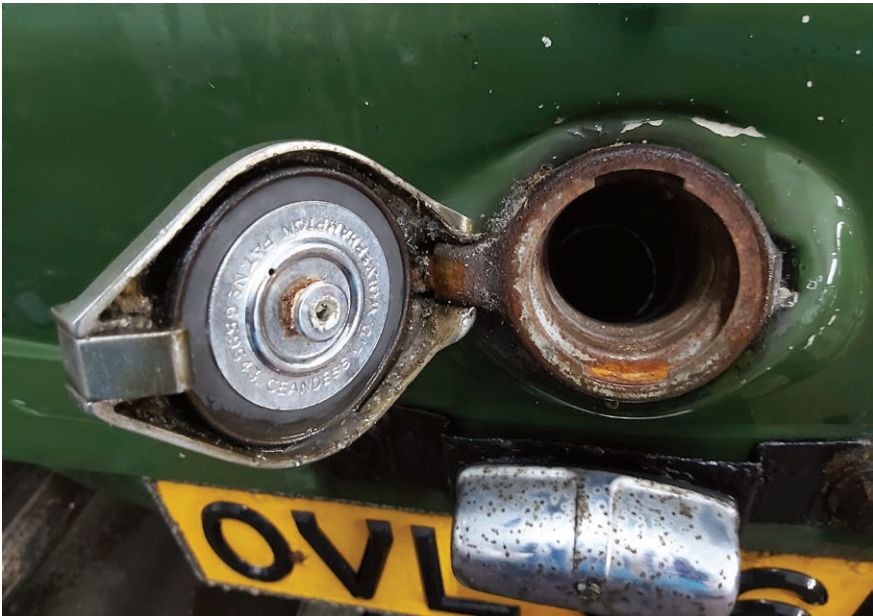
The filler cap at the rear can leak where it goes through the body connecting to the tank. Exercise extreme caution if any fuel smells are present.
