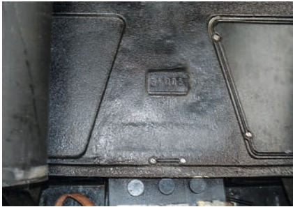
The chassis number is under the mat stamped into the floor of the luggage compartment above the battery area.
