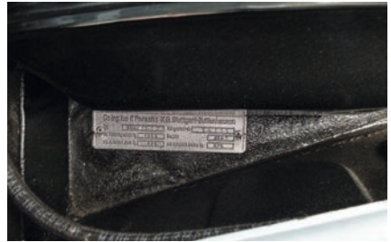
A second ID plate with the chassis number was located to the right of the fuel tank through 1961, and down by the stamped chassis number on later cars.
