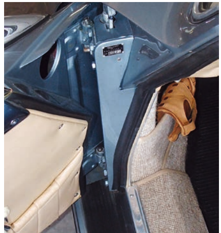
A third coachbuilder plate is riveted to the small aluminium panel that covers the left side door hinges. It also contains the stamped chassis number, and, on some cars, the paint number. On other cars a separate paint plate is below, which may or may not include the paint number.
