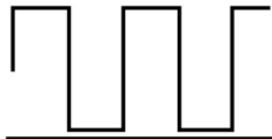
Figure 7-2: A square wave. Note that all of this wave is above the 0V line – this is not an AC waveform.
