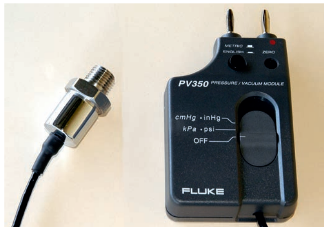
A pressure measuring attachment for a multimeter. Used with a good multimeter, with peak-hold and similar functions, this accessory is very useful.
