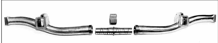
Top: To lower the drive train to the low-mounted dry sump engine and gearbox, the Type 59 rear axle incorporated double reduction gears (primary bevel and secondary spur) within a cast aluminium split housing
