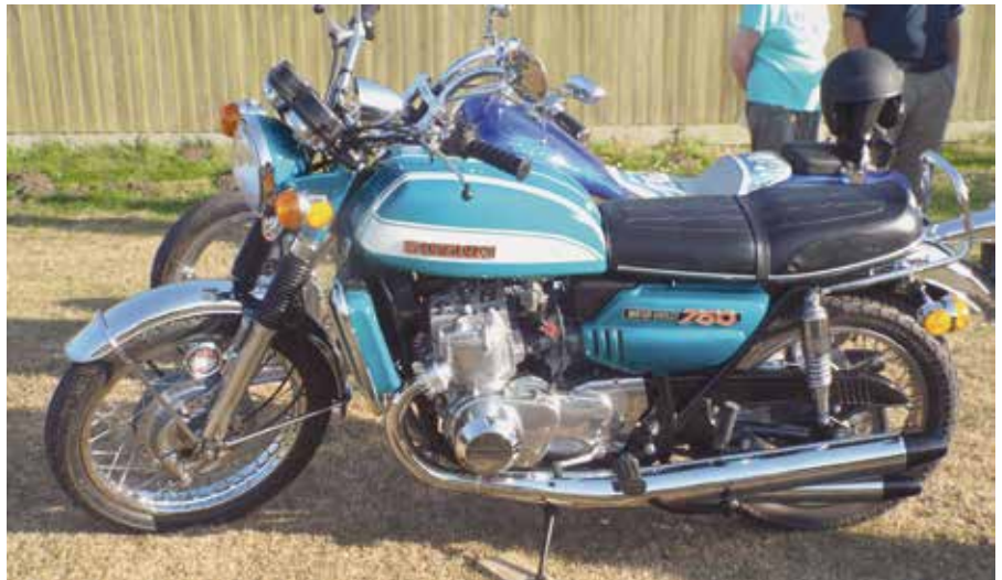
5.0 A Suzuki GT750 water-cooled 2-stroke triple. Originally introduced in 1971, this is recognized as a milestone in motorcycle history, and is the first water-cooled motorcycle produced in Japan to have basically the same engine fitted to the smaller capacity models (the GT550 and GT380); the smaller engines being air-cooled with the aid of Suzuki's Ram Air system.
