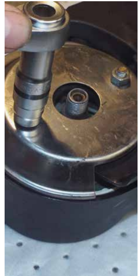
10.20 ... and unscrew the four 10mm nuts to remove the chrome covers.
