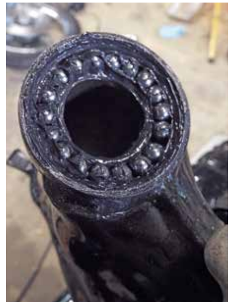
13.18 Put plenty of grease on the bearing carriers when fitting the headstock ball bearings, and make sure the bearings are cleaned and greased before putting them in place. The grease lubricates the bearings, and prevents them falling out while you're inserting the fork stem.
