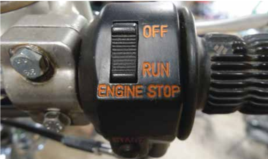
10.17 The switchgear rebuilt, repainted, and looking like new.
