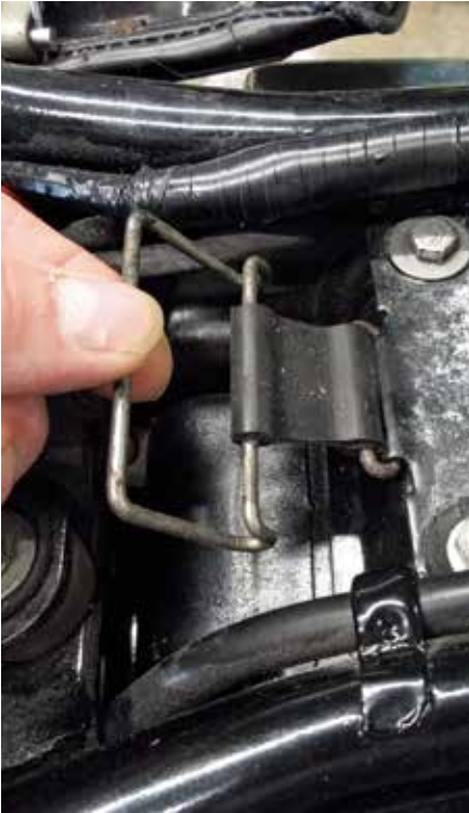
13.15 Some fuel tanks bolt down at the back. On this model an elastic strap is used for quick release.
