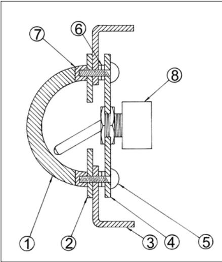
A cross-section of the switch panel installation showing the same features as the previous diagram assembled with spacing washers (6), rivnut inserts (7), and one of the switches (8).
