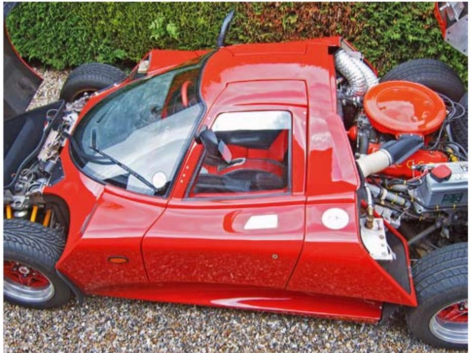
**To make the central body tub every panel had to be modified in some way, much of it being made from scratch.**
