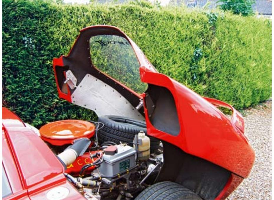
The sheer size of the rear clamshell demanded substantial internal bracing in the form of partitions and box sections.
