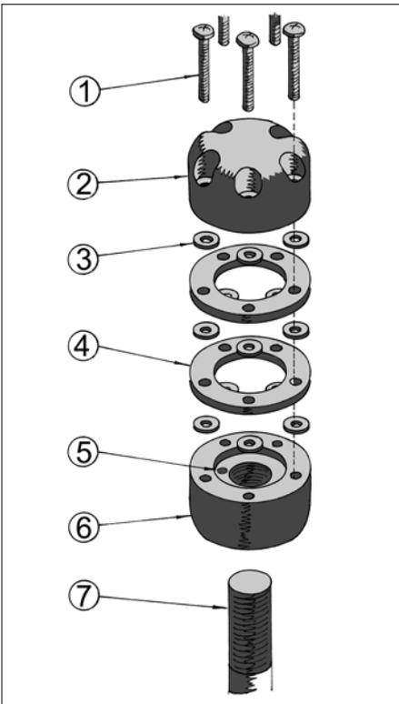
An exploded diagram showing the gear knob construction. The fixing screws (1) pass through the top (2), spacing washers (3) and rings (4) to screw into the base (6). The complete assembly then screws onto the gear lever (7). Note the hole (5) for the power supply wire.
