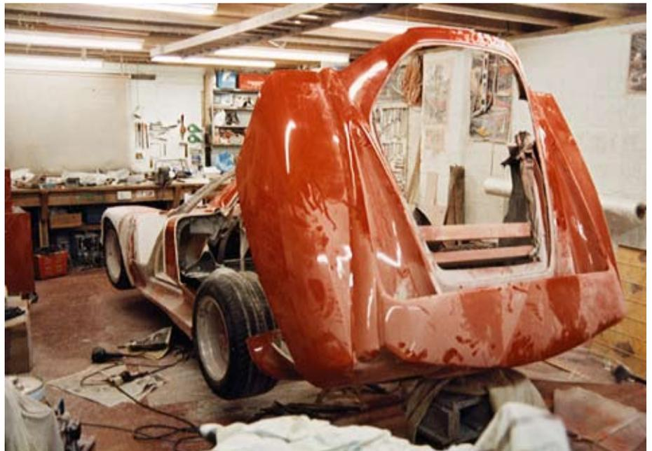
The rear panel cut and hinged open for the first time. Note the wooden bracing across the window aperture, a legacy of the car's mock-up nature.
