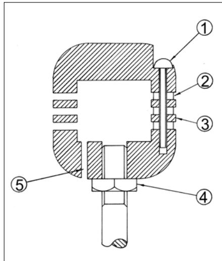
A cross-section of the gear knob assembly showing how the screws (1) pass through the spacing washers (2) and rings (3). The power supply wire hole (5) is located close to the locknut (4) which secures the knob to the lever.
