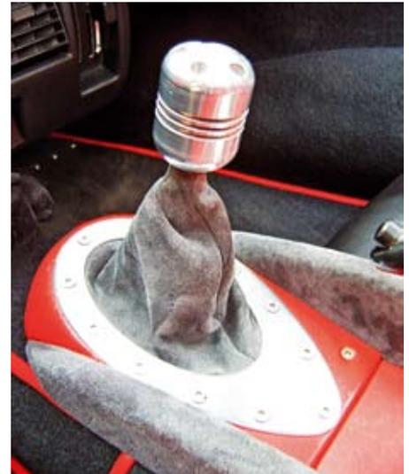
An illuminated gear knob may be a bit over the top. Power supply and earth wires are hidden under the suede gaiter.
