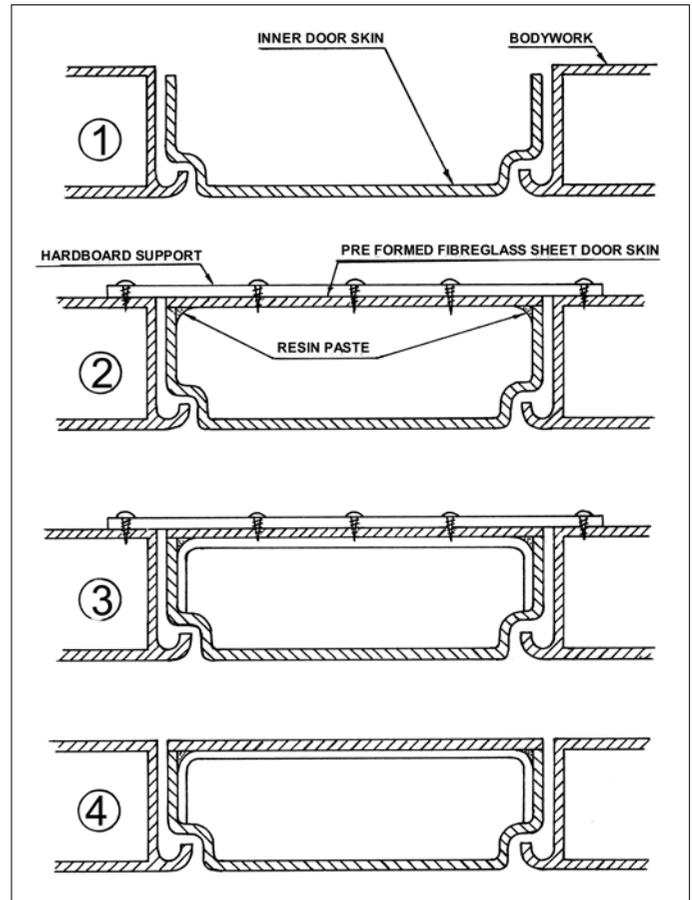
A series of sectional diagrams through a door moulding, showing the process of forming a new door skin. 1) The inner door skin is trimmed to slightly below the level of the surrounding bodywork. 2) Pre-formed fibreglass sheet is held in place with hardboard across the door and bonded with resin paste. 3) The initial bond is augmented with layers of CSM and resin inside the door. 4) The hardboard is removed and the screw holes filled to reveal the new door skin.
