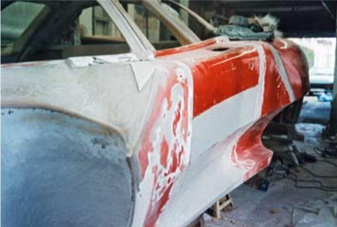
The hardboard has been removed to reveal the new door skin, which follows the complex shape of the side of the car.
