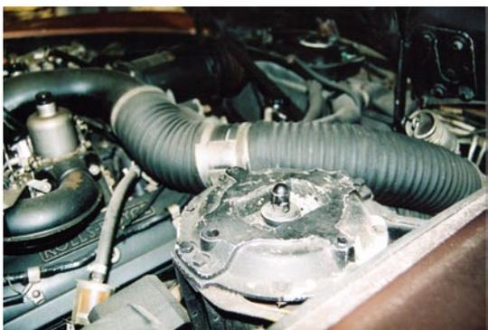
**Under-bonnet trunking should not be split or damaged.**
