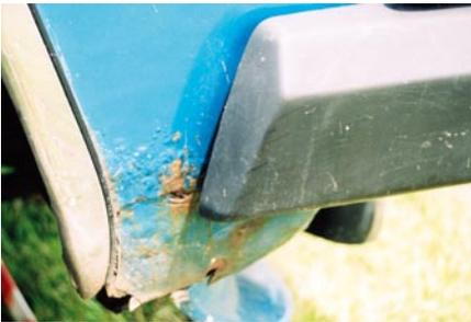
Advanced corrosion along the lower flanks of a car could be a reason to walk away from a deal!
