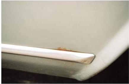
Look for evidence of even minor corrosion which, left unchecked, can become serious.
