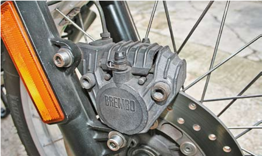
Lack of use can result in sticking pads and dragging brakes.
