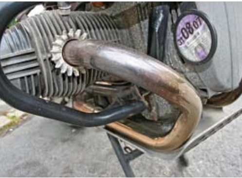
The downpipes and silencer last well.
