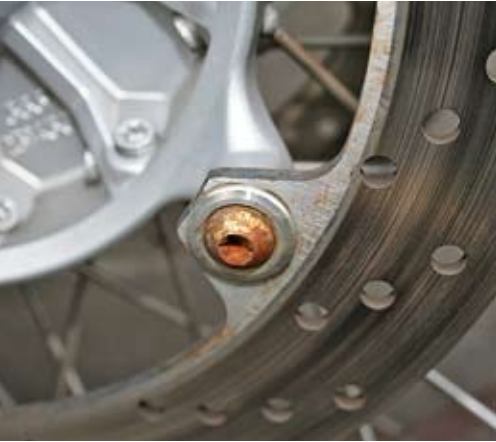
Rust attacks damp metal.
