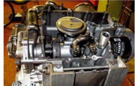
**Fig 3.4 Oil pump pick-up, strainer and relief valve.**
