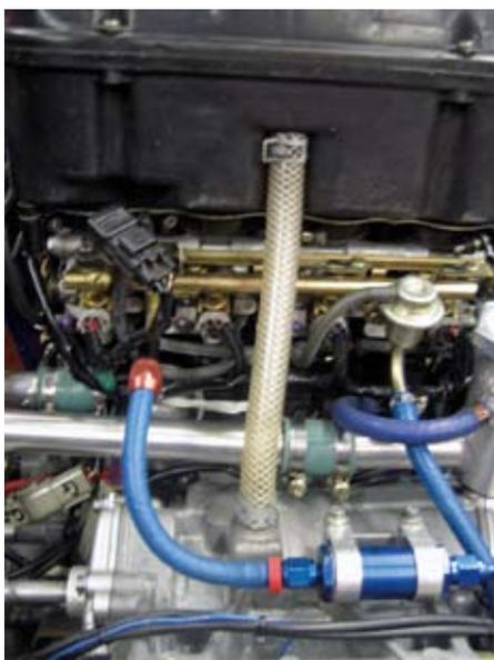
**Fig. 13.3 Fuel-injection system showing injectors (red wires attached), fuel rails, dump valve (to right of centre), and engine breather discharging to airbox.**
