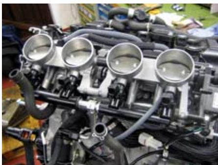
**Fig. 13.4 Fuel-injection throttle bodies.**
