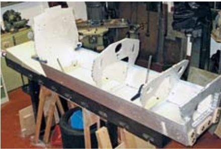
Fig. 8.11 'Dry' fitting of bulkheads.
