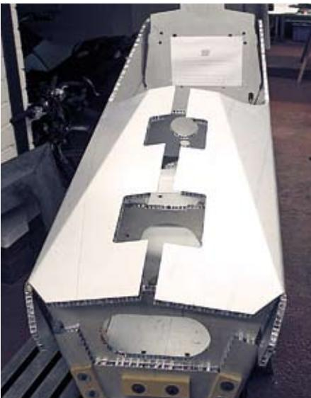
Fig. 8.12 Dummy run of monocoque folding.
