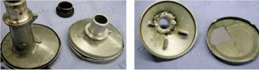
**Fig 3.3 Original (left-hand) and modified oil pick-up strainers.**
