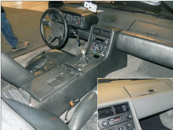
**Left: a black interior five-speed car, note the separate digital clock fitted just in front of the gear lever, and the aftermarket stereo.**
