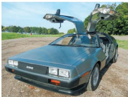
**The doors should stay upright without assistance, if not, check the gas strut before attempting any other adjustments. The front amber marker lights on the wings/fenders can be modified to also act as indicator side repeaters – a wise modification.**
