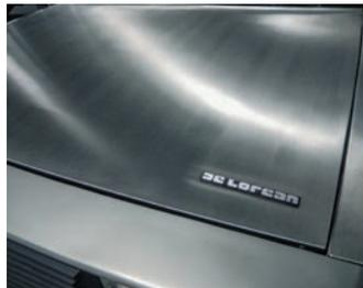
**Left: the first DeLorean hoods/bonnets were produced with both a fuel filler flap and grooved 'accent' lines running down each side. Centre: the mid-style hood with the omission of the fuel filler flap, but retaining the grooved 'accent' lines down each side. Right: the final variation of hood, completely flat with an additional raised DeLorean badge on the front corner.**
