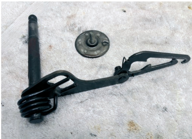
29.4 The gearchange shaft and pawl mechanism.
