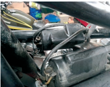
7.6 Ignition coils in situ under the tank.
