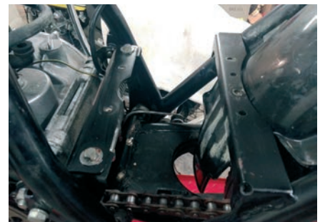
7.12 Battery carrier assembly removed.
