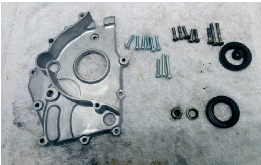
29.6 Gearbox casing with set screws and seals ready to be inserted.
