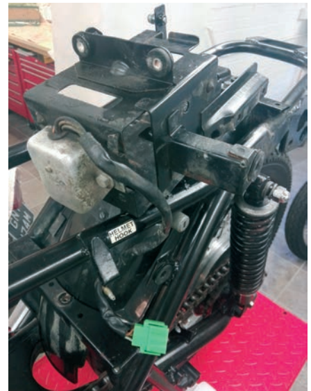
7.11 Rectifier bolted to bottom of battery carrier.
