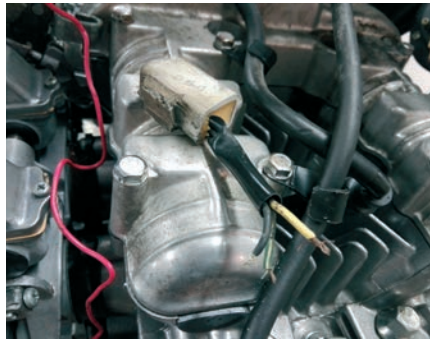
7.8 This strange unit had been disconnected and left hanging – but what was it? (The rear brake light failure switch, it turns out).
