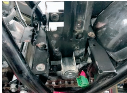
7.9 Left-hand side of battery carrier assembly before dismantling.
