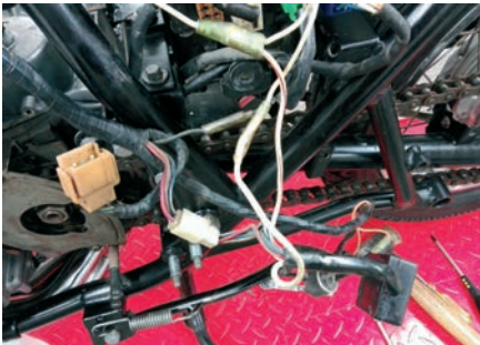
7.5 Main electrics being stripped out.
