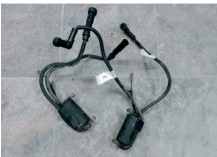
7.7 Ignition coils removed and labelled.
