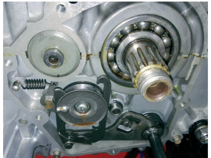
29.5 Gearchange shaft in place, along with the 'O' ring on the main shaft.
