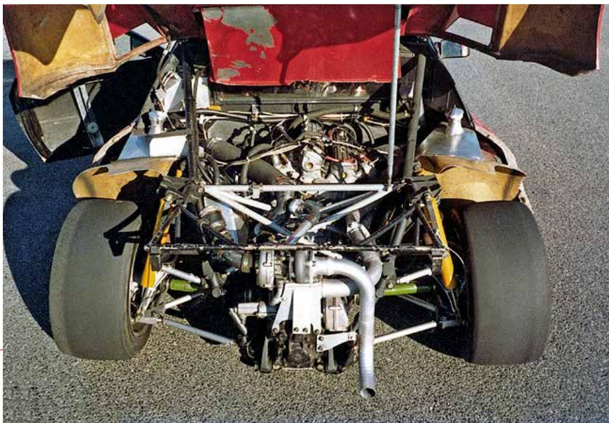
*Developed by Tonti at Lancia's Via Caraglio workshop, this is a 1750cc turbo engine fitted to 001.*
