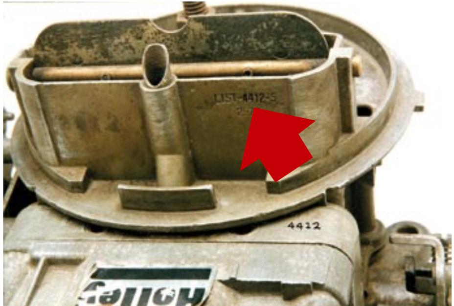
**The two barrel Holley carburetor List Number is found on the choke tower. Relevant numbers on this particular carb are 'LIST-4412-S' with '4412' being significant numbers making this particular carburetor a 500CFM one. The numbers 2572 underneath are not relevant to the identification of the carburetor, just the top line after the word 'LIST.'**
