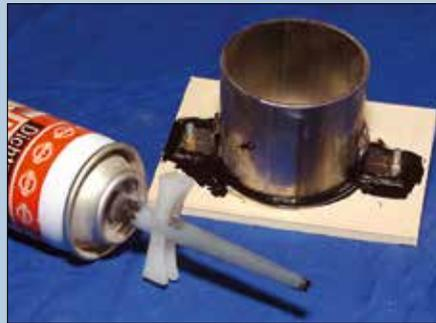
The most important thing is that it should be tightly sealed (here using silicon sealant), so that the moulding compound cannot leak out.
