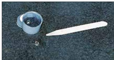
The fibres are thoroughly mixed together with the metal ball in the mixing tin.
