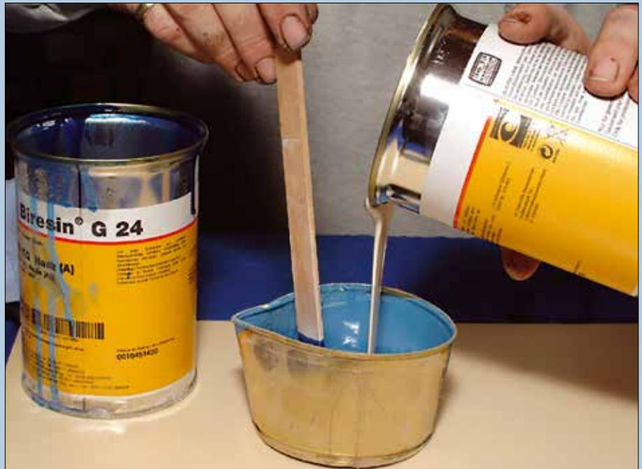
The moulding compound is mixed in equal parts with the hardener and thoroughly stirred together.
