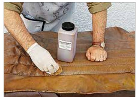
The base coat is rubbed into the leather by hand. Subsequent coats ...
