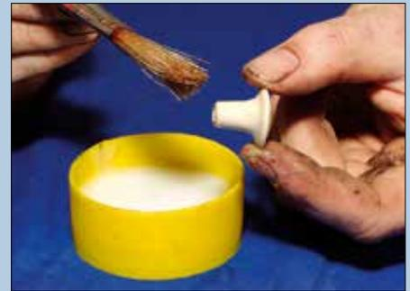
Keeping things apart: release wax is brushed onto the original part, so that the moulding compound ...
