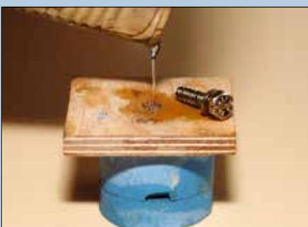
The original is removed at the separating line, and the cavity filled from below with synthetic resin.
