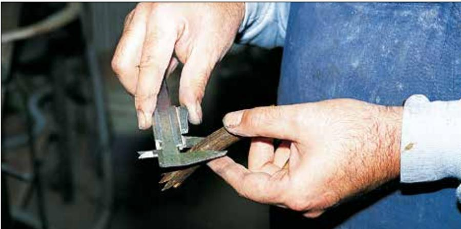
The thickness of the old wood sets the measure for the restoration. Many customers take the opportunity to make the thin rim of their steering wheel a little thicker. Just an extra millimetre can make the wheel noticeably better to hold.
