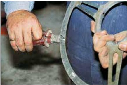
The old rivets are simply nipped off with a pair of pliers and then ...
