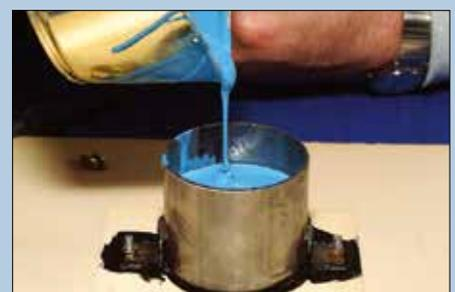
The cover is now poured in above the separating line formed by the release wax.
