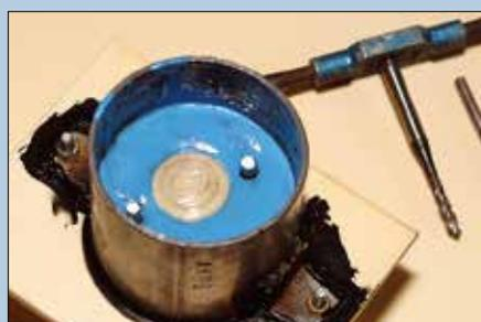
After the compound has dried, two locating pins are inserted, then everything is coated with release wax again.
