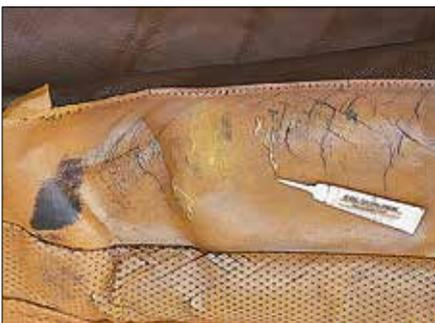
Small cracks are also filled: in this case, with liquid leather filler from a tube.
