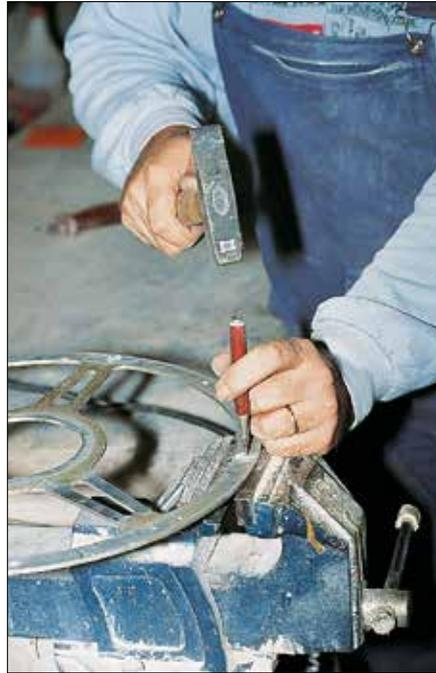
... knocked out with an awl. The rim should be supported as shown here, or it will buckle.
