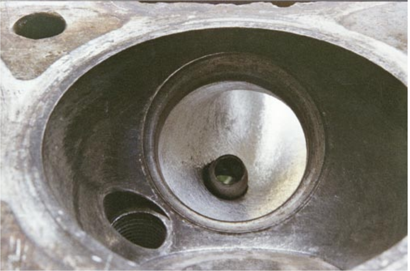
The original valve guide was removed before work commenced. The port has been roughed out with a rotary file and a new valve guide fitted. The valve seat is still standard.
