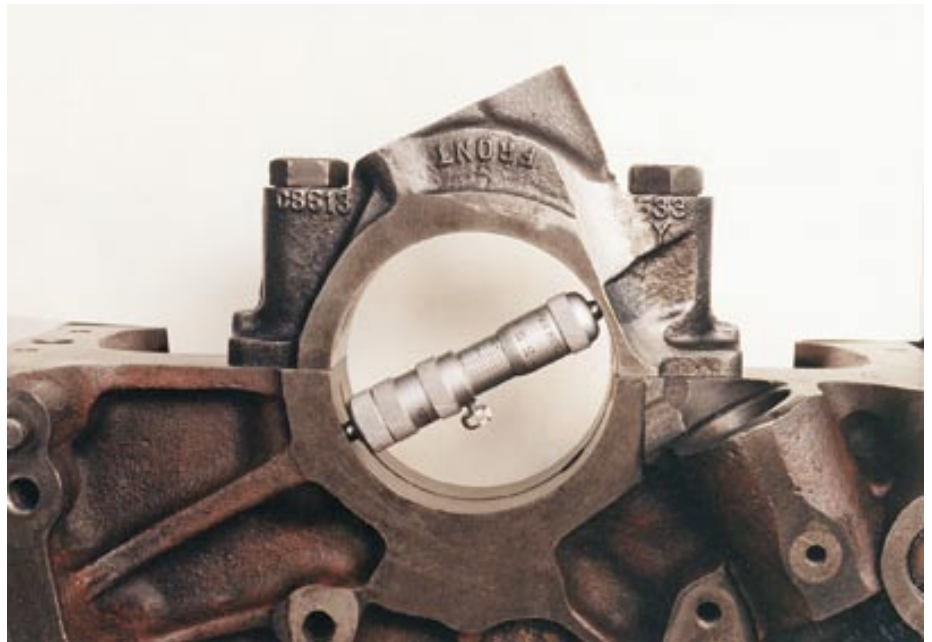
Main bearing tunnel being measured in the second position ...
