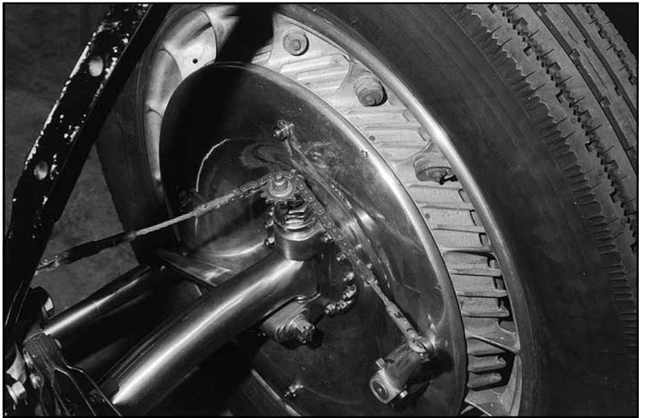
in fact, follow very closely that of the Type 41, including the transmission arrangements aforementioned, incorporating a three-speed gearbox in the rear axle. Rudge wire wheels were specified in place of the magnificent aluminium type designed for the Royale, although another elegant wheel was conceived for the later Type 50 which became available as an option for the Type 46. Several earlier cars were retrospectively converted.
