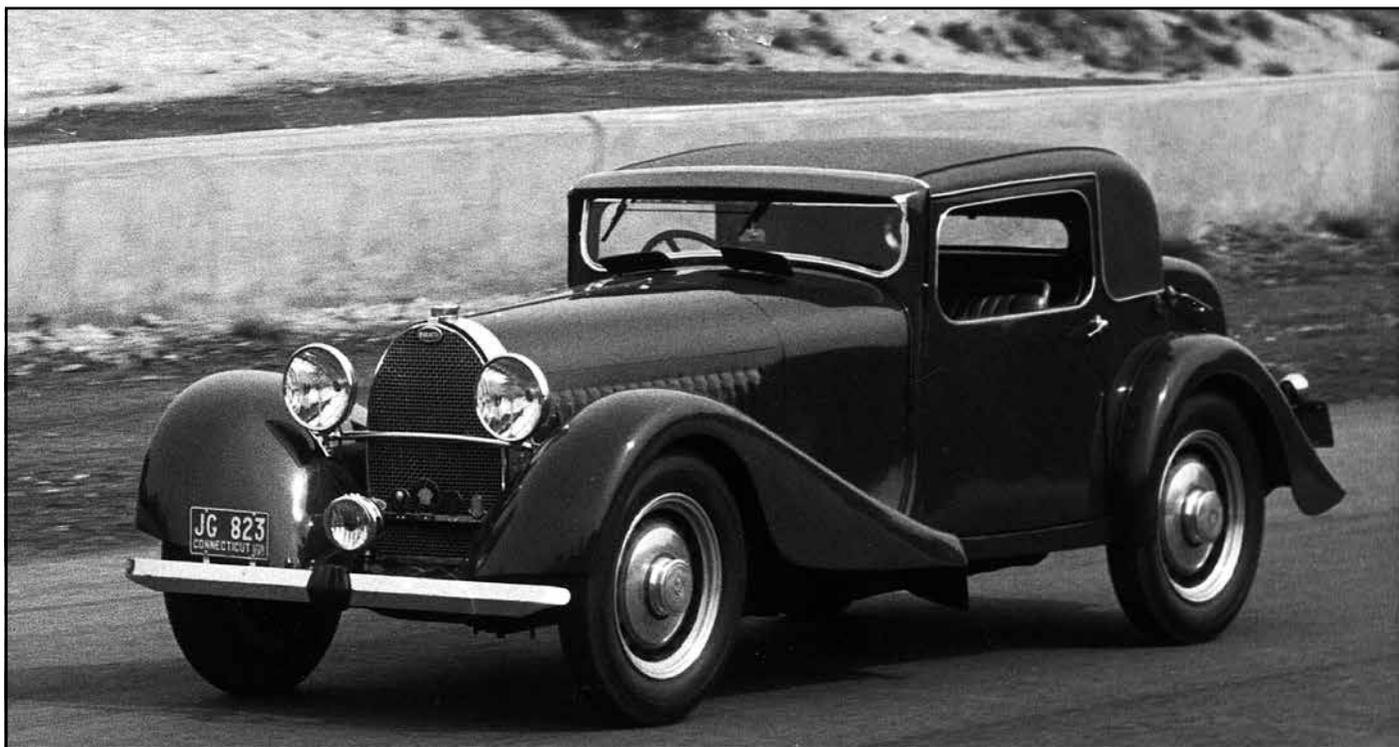
*Type 50. Short chassis, 2-door Saloon by Million-Guiet. This body was heavily modified in the forties, but is now being restored to original state.*
