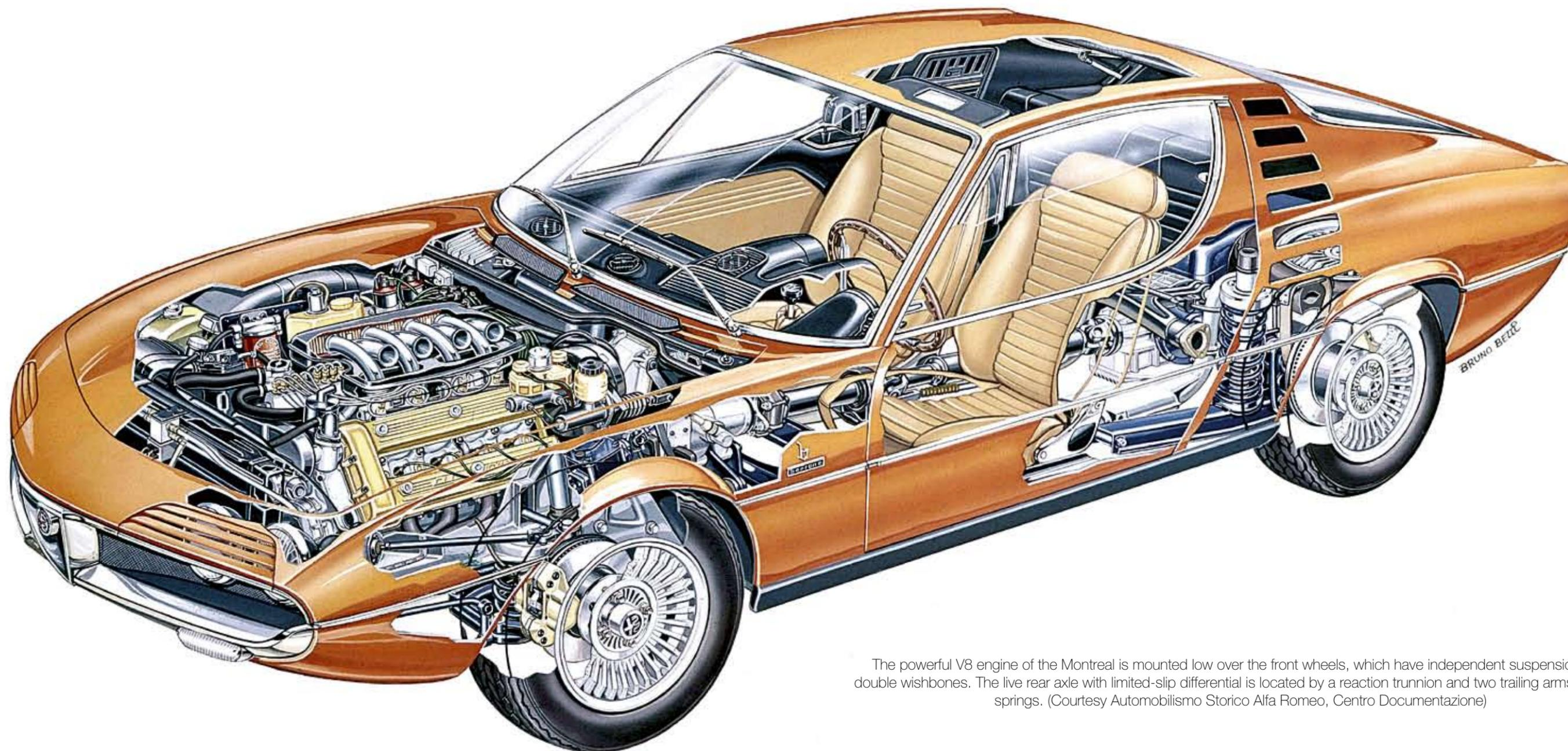
The powerful V8 engine of the Montreal is mounted low over the front wheels, which have independent suspension with double wishbones. The live rear axle with limited-slip differential is located by a reaction trunnion and two trailing arms with coil springs. (Courtesy Automobilmismo Storico Alfa Romeo, Centro Documentazione)
