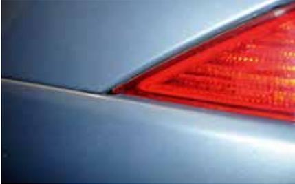
**Ensure rear light units are not damaged, as the edges are sharp and easily cracked if they have been previously removed.**
