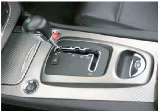
**The J-gate style transmission system of the 4.2-litre engine models.**
