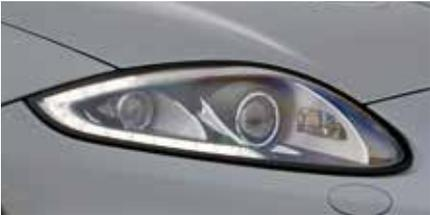
**The later type light units fitted to XKs from 2011. A totally different design, incorporating running lights.**
