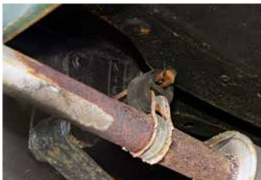
Exhaust hanger positions reveal an Escort's identity, this being a stock non-RS Mk2 setup.
