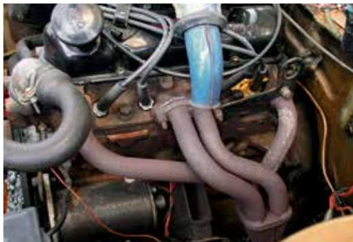
GT-spec Crossflow engines had a tubular exhaust manifold, prone to cracking on the welds.
