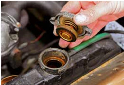
Remove the radiator cap when cold to check the colour of the coolant.
