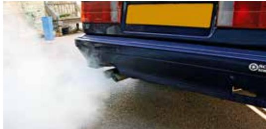
**White water vapour when starting a cold engine on a cold day is normal, but grey or blue smoke indicates possible engine wear. Whilst looking at the back check the lights, lock and boot for corrosion.**
