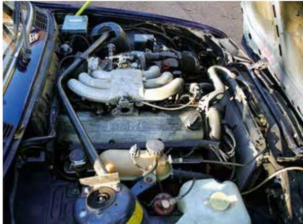
**What's the general impression? Leaks and spilled fluids are signs of poor maintenance. Equally, if the engine bay has been pressure washed it may indicate an attempt to hide leaks.**
