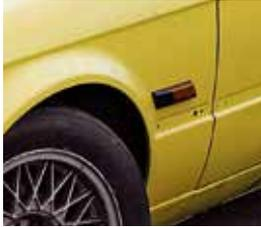
**Check that all the trim parts are present and secure. This car has missing rubbing strips, which are getting harder to find in good condition.**
