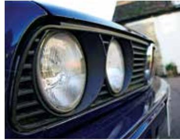
**Check that the lights work and that there isn't moisture residue inside the lens. Look through the grille at the integrity of the radiator. Check that the front bumper and trim is secure.**
