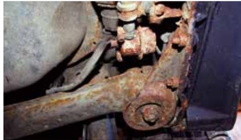
**This fuel pump assembly is corroding and its mounting brackets are weak. Check all components underneath if the car has stood for a long time.**
