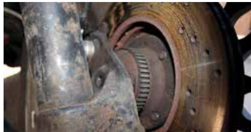
**This brake disc has light surface corrosion due to being static for a few months. If corrosion was any more severe than this, the disc would need to be resurfaced or replaced.**
