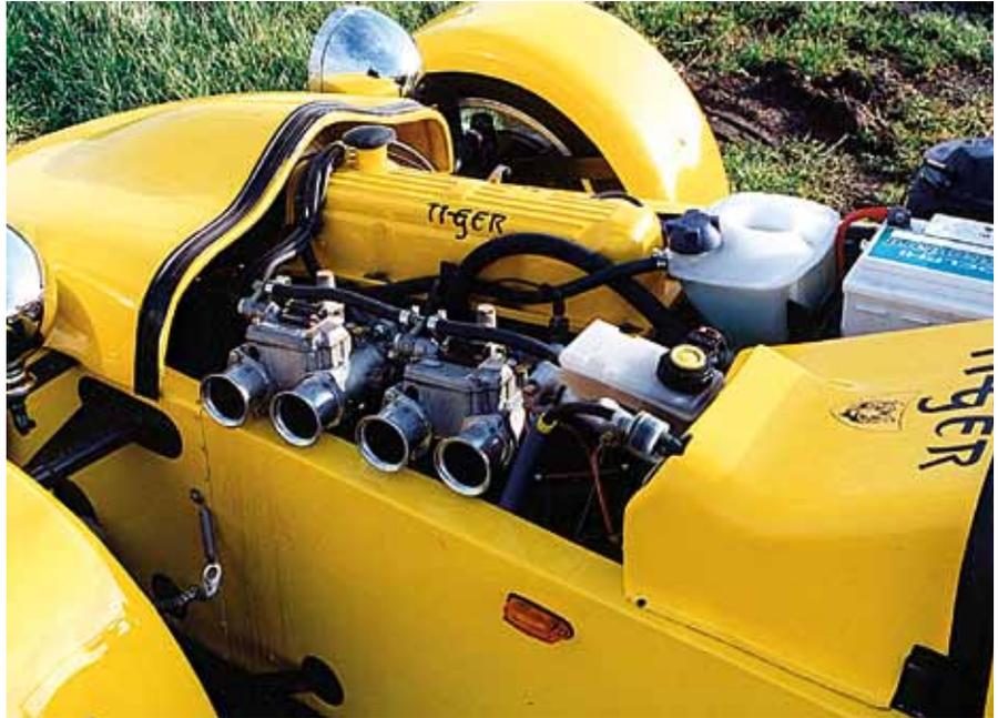
Left-hand drive Tiger Cat with Ford SOHC 'Pinto' engine (fitted with sidedraught carburetors).
