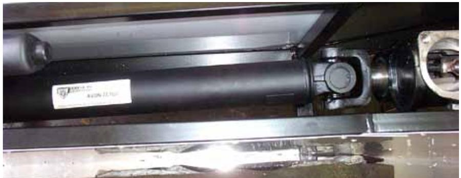
New Tiger Avon propeller shaft. Note the distance on the sliding part of the prop, between the oil seal and the U/J: this is to allow for movement of engine and gearbox mountings.
