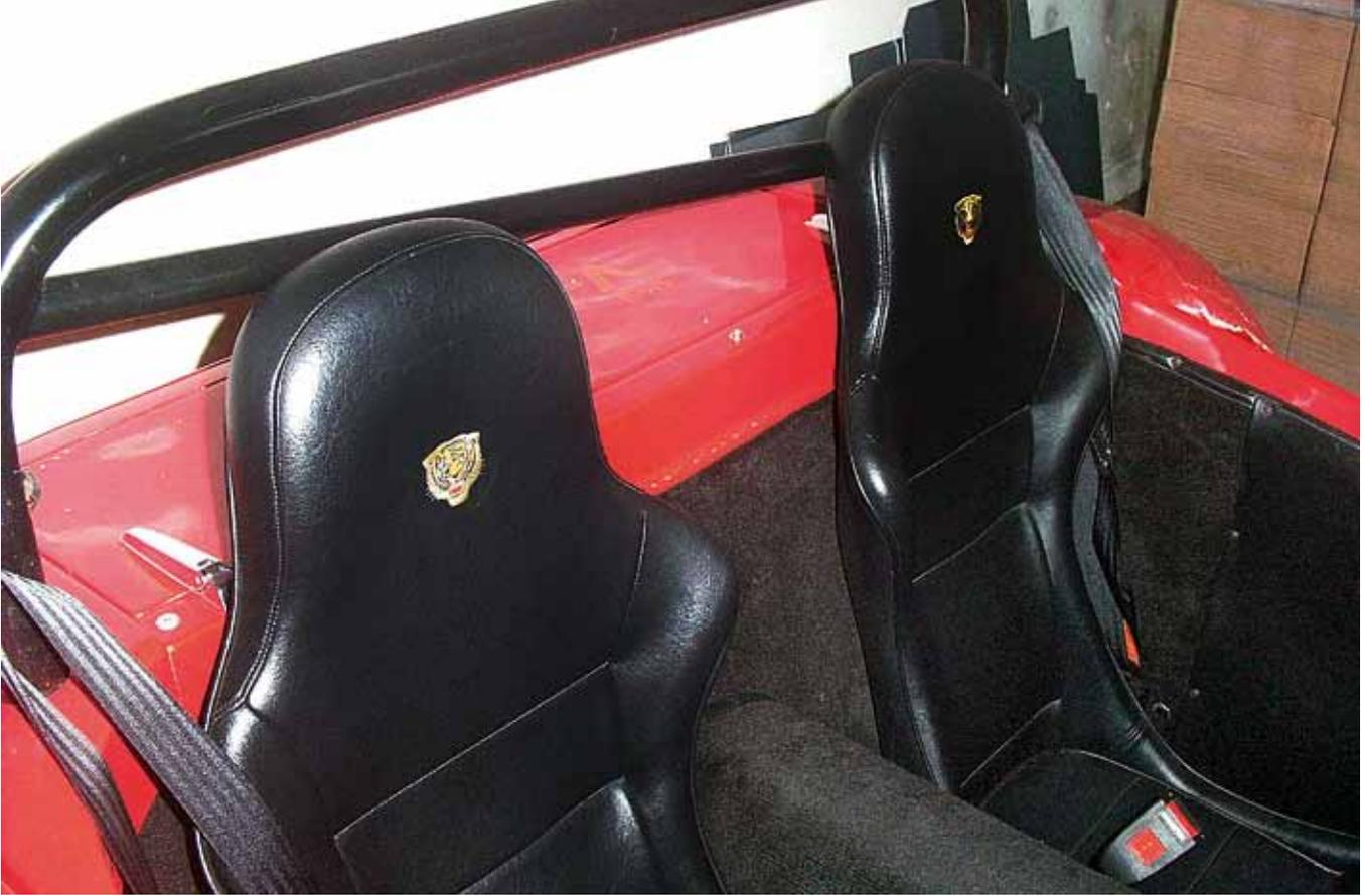
An example of a high-back seat: this type of seat or individual headrest is required for IVA.
