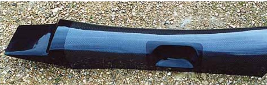
Tiger R6 carbon fibre transmission tunnel.
