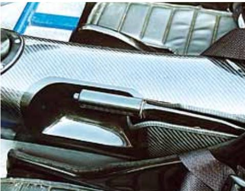
Handbrake (parking brake) area detail of a carbon fibre transmission tunnel installed in a car.
