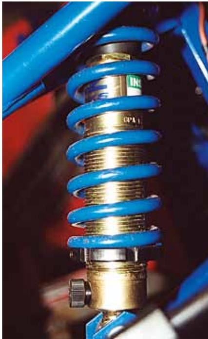
**Telescopic suspension unit with adjustable damping (resistance) and a spring platform adjustable for height.**
