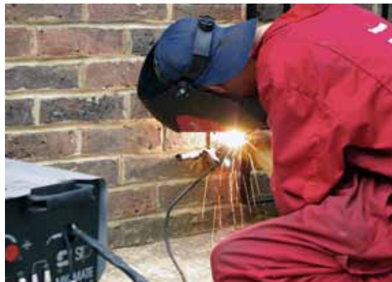
18-11. Gasless MIG is well suited to outdoor situations.
