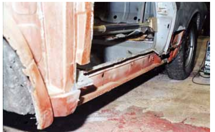
8-28. Original red oxide is a good sign. Note expanding brace.
