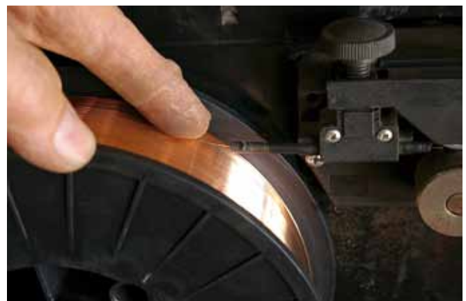
18-12. Reel of copper-coated 0.6mm wire.
