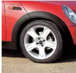
**Above: Bullet-style 17in alloy wheels fitted to face-lifted R50 Cooper and Cooper S models. (Courtesy MINI UK)**
