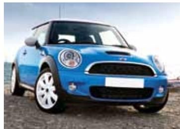
**The second generation R56 MINI Cooper S, introduced to all markets, was turbocharged rather than supercharged. (Courtesy MINI UK)**
