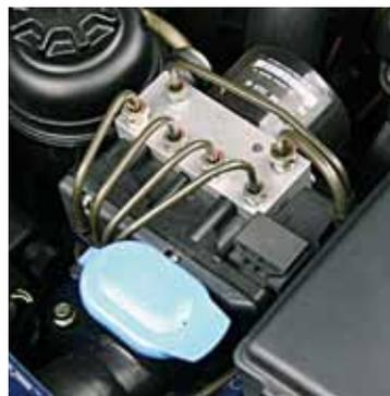
**ABS modules are expensive to replace, although they can now be repaired.**
