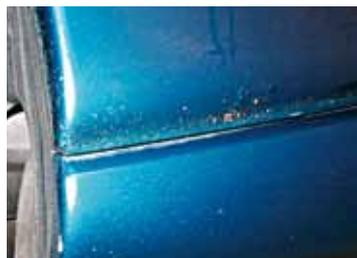
**Minor corrosion in an older car is normal and not a major issue.**
