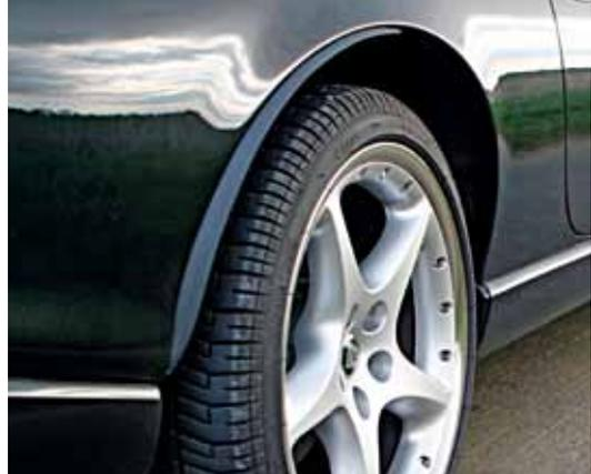
**Rubber wheelarch extensions should always be fitted with the bigger rear wheels.**
