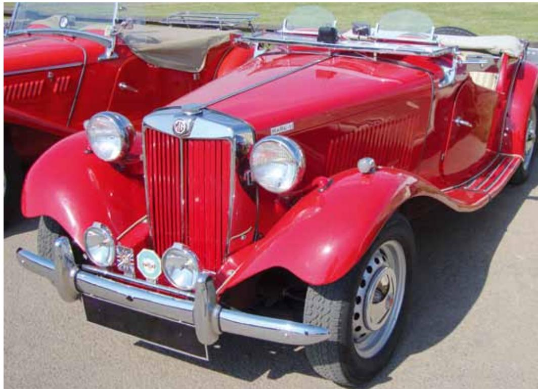
This rare TD Mark II has a good radiator shell and the correct front bumper and over-riders. You can also see the alloy metal strips on the running boards, with rubber inserts.
