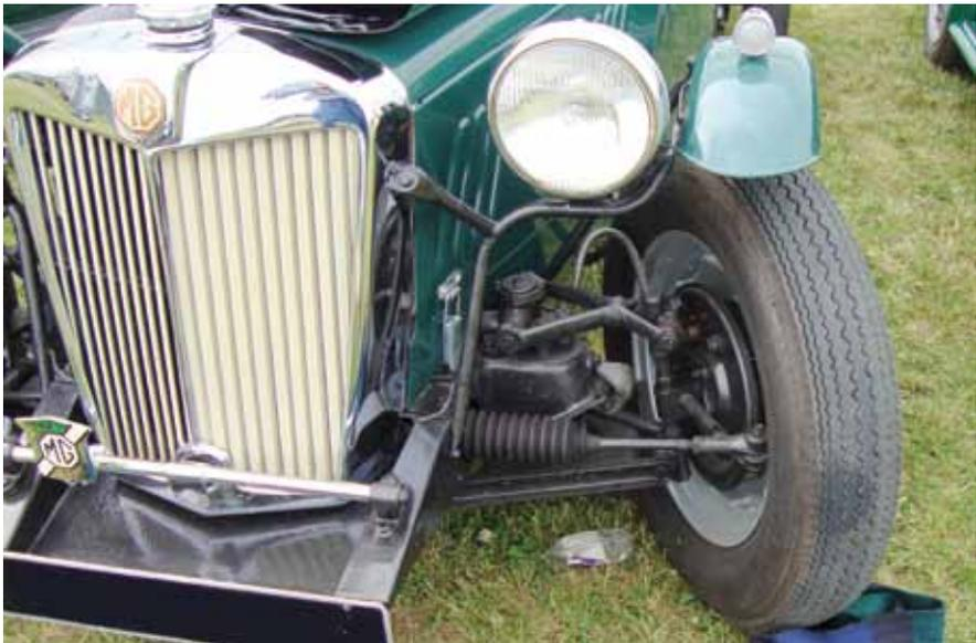
A TD fitted with non-original cycle wings, clearly showing the early type of TD shock absorber.
