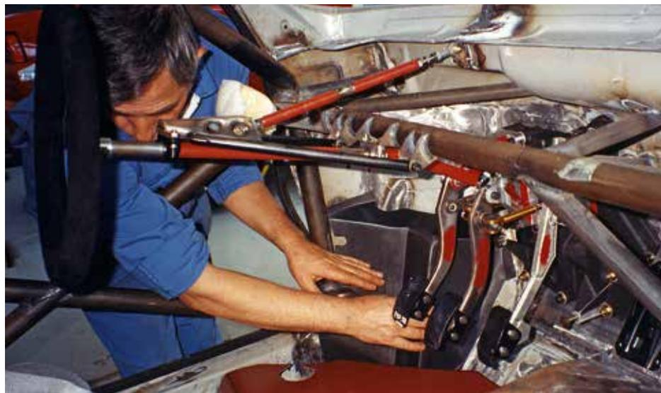
Inside the '94 car during the build process. Note the support for the long, raked steering column.
