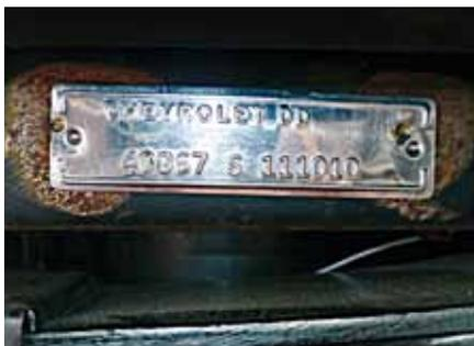
The vital VIN tag; spot-welded on the bar below the glovebox on this 1964 car.
