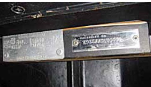
Trim and VIN tags both retained by rose-head rivets in 1965-1967 cars.
