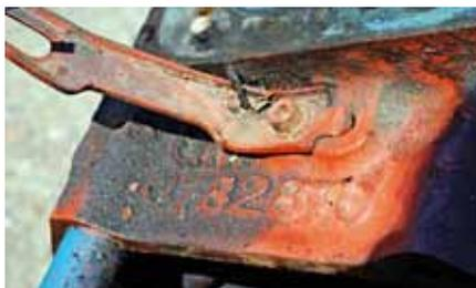
The cast number on the back upper left hand of the engine block. 3782870, seen here, was used in almost all small block Corvettes from 1963-1965.
