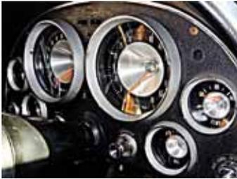
**1963 gauges used cranked needles and deep conical silver faces.**
