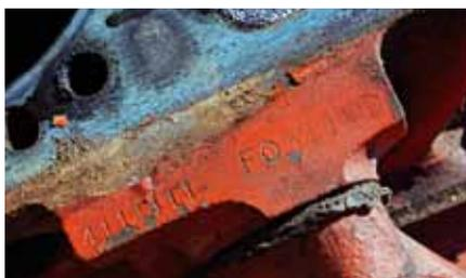
On a 1964 car, 4114411 was the VIN derivative stamped at the St Louis assembly plant, while FO311 RD was stamped at the Flint MI engine plant. Flint usually used capital letter 'I' to represent the figure '1,' and RD denotes 327-300hp assembled with a manual transmission.
