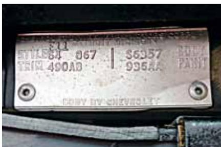
The Trim tag shows information about body colours and date, seen here riveted in a 1964 car.
