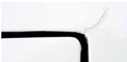
Cracking in the body at the headlight opening is a badge of honour; indicating a Sting Ray that has been driven, not stored.
