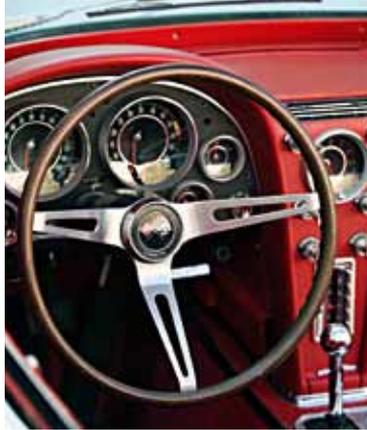
**1964 gauges are still conical, but with black centres. Air-conditioned cars have an extra vent and control knobs above the clock.**
