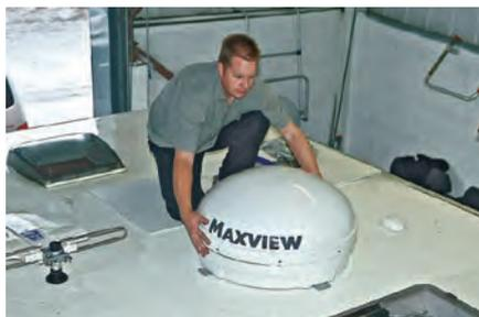
Picture 1. Adventure Motorhomes' Nick Stevens started by positioning the new dome on the centre of the roof. He then marked the position of each of the mounting points on the roof ...
