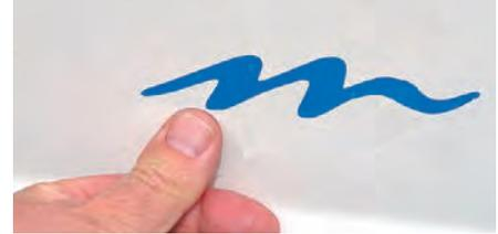
Picture 8. ... and wetting the graphic prevents the self-adhesive layer on the back of the graphic sticking to itself. Slide the graphic (which often consists of separate parts) onto the paintwork. Don't worry, it WILL stick when the water dries.
