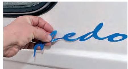
Picture 9. The main section of this particular graphic is being placed on the panel. It will slide around very easily, but keep your fingers wet, too – it makes it much easier to handle!
