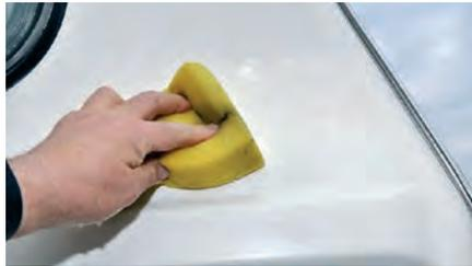
Picture 6. Fitting a graphic is a similar process. Because of its size, it's much more likely you'll trap air bubbles. So sponge some soapy water onto the panel. While still wet ...
