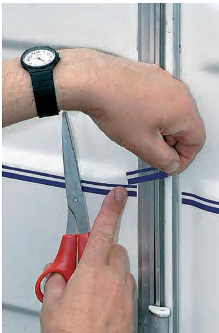
Picture 5. As you saw earlier, you go right over door and access hatch openings, then go back later and carefully cut to fit. Some favour a sharp knife – but don't scratch the paint.
