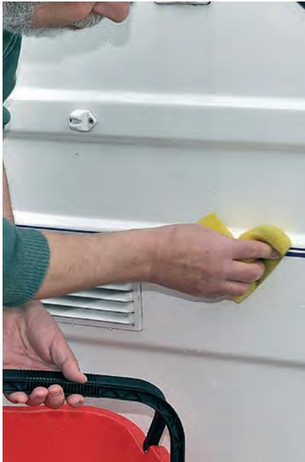
Picture 4. ... before pressing down lightly. Do one or two metres at a time, and don't press down TOO hard until you're sure it's positioned correctly. Use a wet sponge for the final smoothing.
