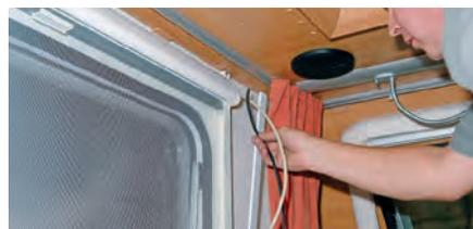
Picture 4. Inside, Nick had already calculated a wiring route through wardrobe, lockers, and bed boxes, but needed to add self-adhesive white plastic cable trunking alongside one of the window blinds.
