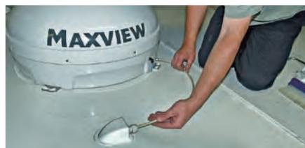
Picture 5. Maxview provided a waterproof access point for the cable on the roof, held down with double-sided tape. You may need longer cable, depending on where you locate the dome and TV.
