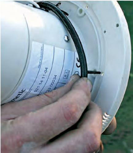
Picture 5. The Dometic vent unit came with its own neoprene seal that had to be fitted in the sealing groove around the base of the top flange on the unit.
