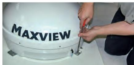
Picture 3. Nick drove stainless steel screws through the mounting holes, having first put a dab of sealant into each hole so the screw thread sealed itself. Be careful: the aluminium is thin.
