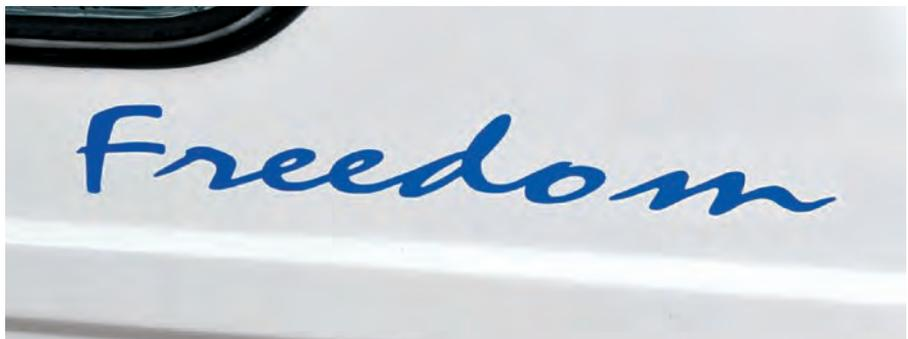
Picture 10. It's vital that you spend time aligning the graphic correctly, AND that you squeeze all air bubbles out. For larger graphics, use a squeegee, removing air gently from the centre, outwards.
