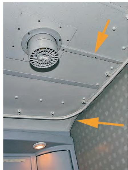
Picture 10. The fan body protruded slightly: if you haven't enough head room, plan to fit it to one side. The wiring was neatly trunked to the ceiling (arrowed).
