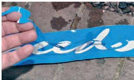
Picture 7. ... and after peeling the vinyl graphic off the backing paper, get ready to place it on the panel. It's best to wet the graphic before peeling: it will inevitably wrap around on itself ...
