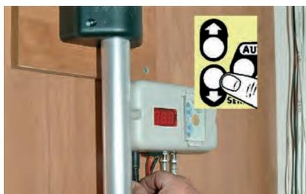
Picture 9. Next, power and antenna cables were connected to the control unit. One button raises the dish to the exact required elevation; another folds it away again.
