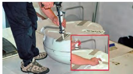
Picture 2. ... before thoroughly degreasing both the roof, and all of the mounts. He then gunned a top quality adhesive over each mounting point, and repositioned the dome accurately on the roof.
