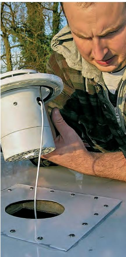
Picture 6. Fitter, Dave, added two strips of butyl sealant. Caravan manufacturers use this to seal some joints, and it never sets, allowing removal in future if necessary.
