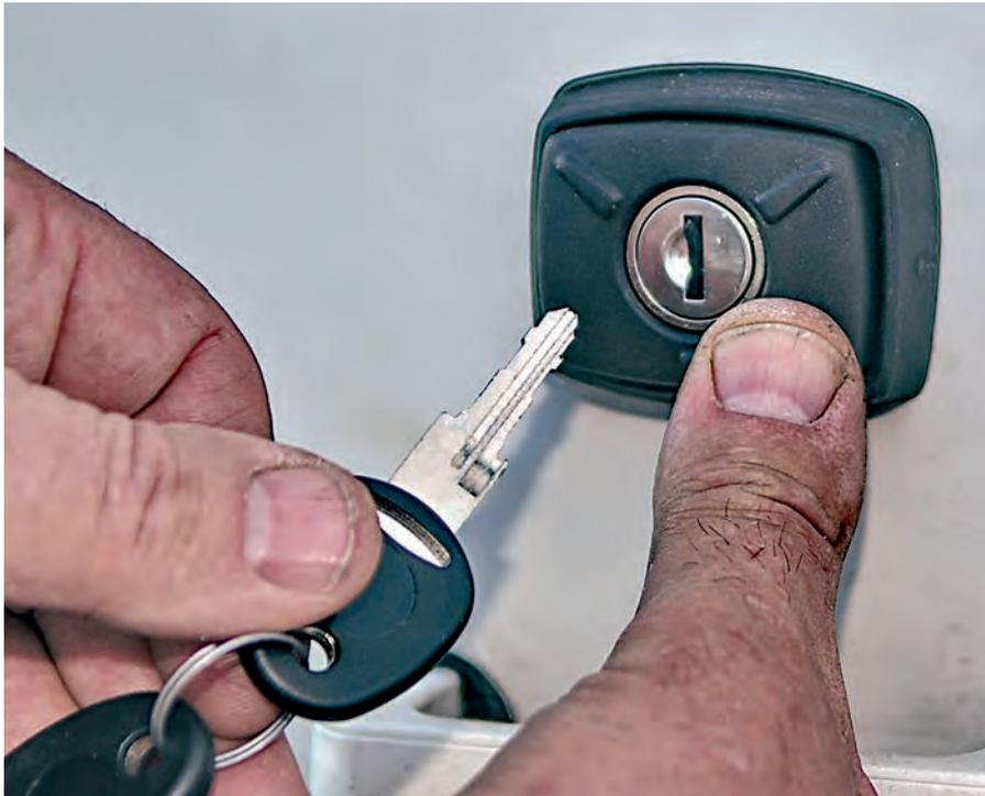
Picture 1. On this fibreglass (GRP) caravan, the locker lock broke, and we couldn't find a like-for-like replacement. It was simpler (and probably cheaper) to remove the old lock and fit a standard item, for which replacement keys could be found if necessary. We used a version from CAK.
