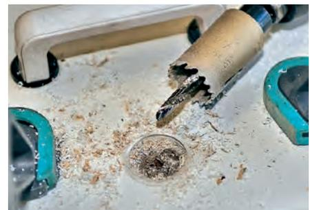
Picture 5. The piece of wood was used because a hole cutter (used to make the larger hole) can't enlarge an existing hole unless there is something to support the centre of the bit.
