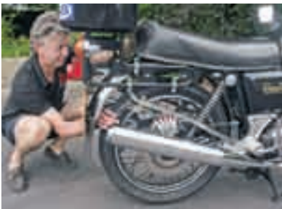
With the bike on its centre stand, check for play in the wheel bearings.
