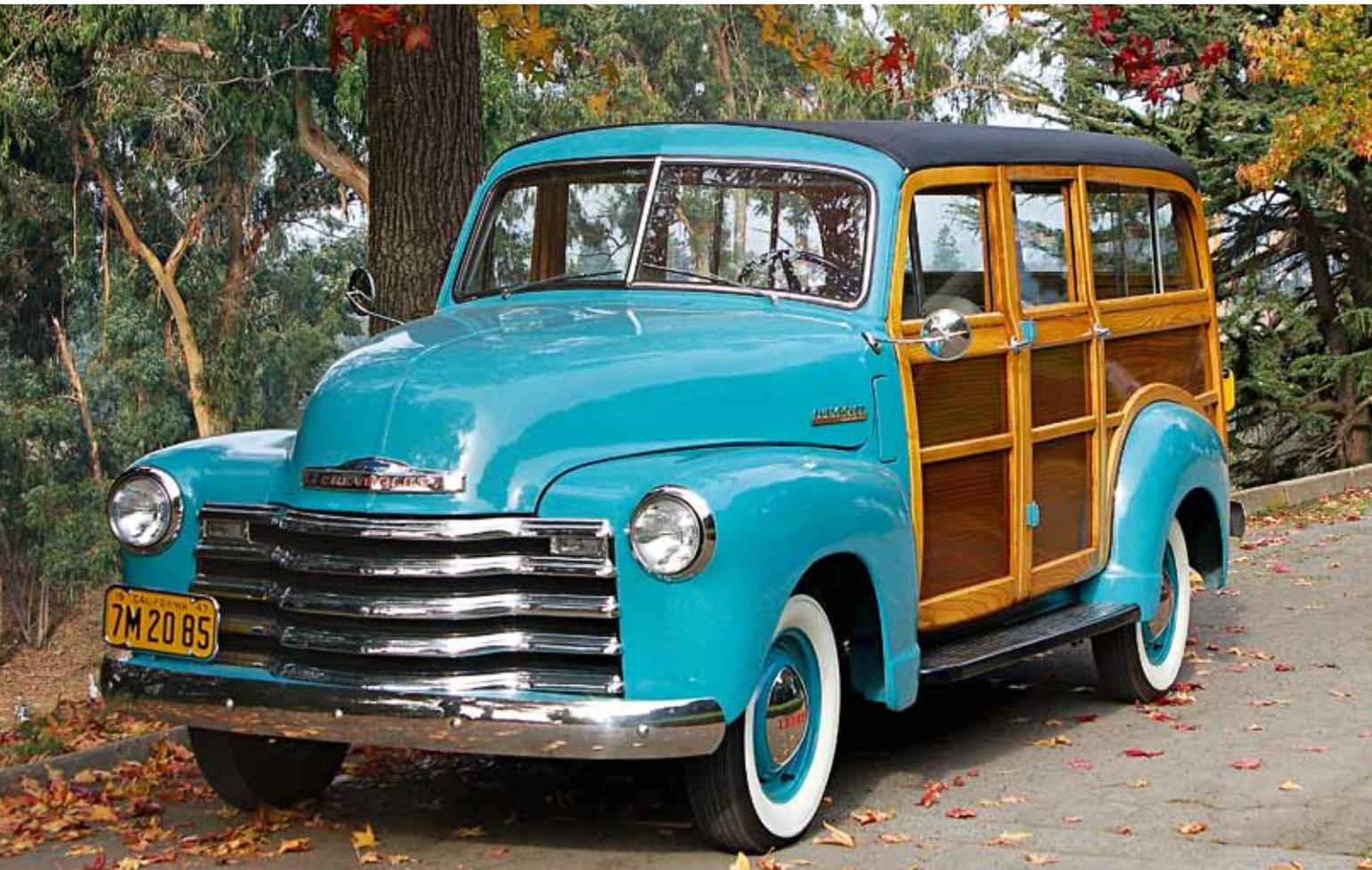
This 1947 Chevrolet Suburban woody was built on a ½-ton, 116in wheelbase Carry All and pickup chassis, and powered by a 216in<sup>3</sup> (3.5L), 90hp, six-cylinder engine. Cantrell was the builder and its special order woody bodies were actually available through to 1955 for GMC, Chevrolet and Dodge truck chassis. (Courtesy Don Bryant)
