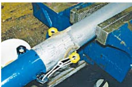
If a rock hits the silencer, this can spring apart. The exhaust will hit the ground with far less damage, and engine rock is absorbed thanks to supreme flexibility.
