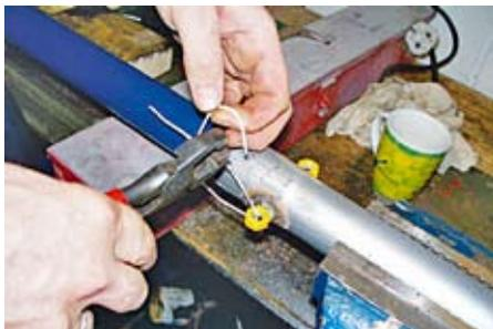
Coat hanger wire is now run through the nuts, in a figure of eight.
