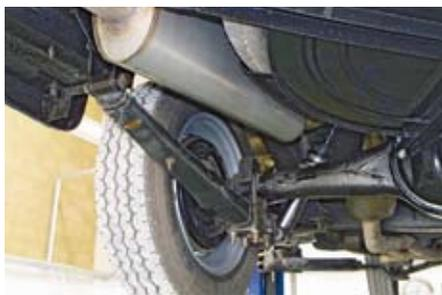
This Riley Pathfinder has the exhaust nicely tucked up out of the way – getting at the spare wheel could be a hassle ... nuts under the leaf springs look vulnerable.
