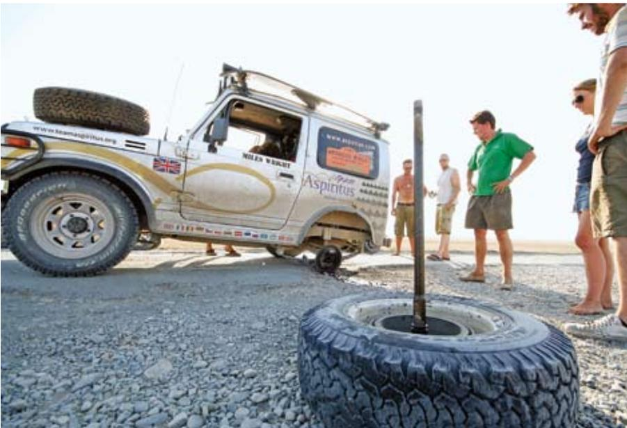
**Suzuki with broken halfshaft – an over-heavy, wider tyre added to the strain.**
