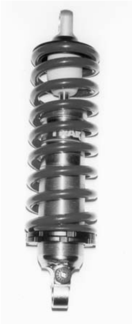
Typical coil-over shock absorber.
