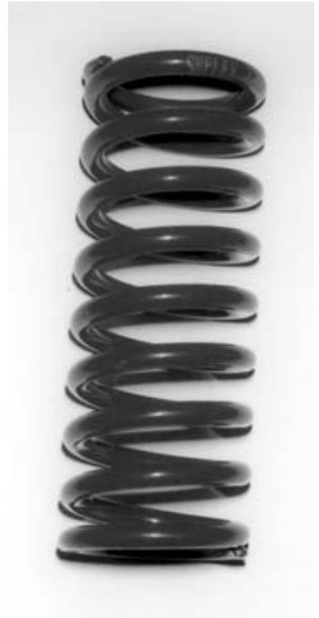
Typical coil spring for a coil-over shock absorber unit. Poundage is always marked on the spring. If it isn't, get it checked for rate.
