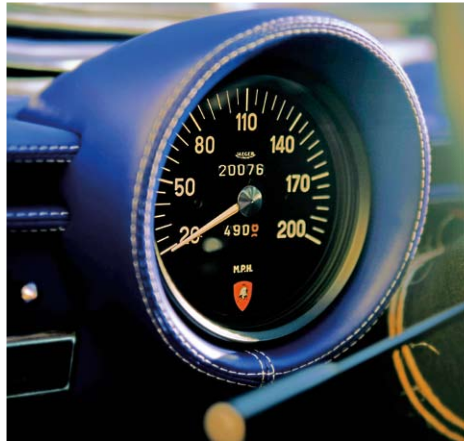
First series USA-spec SVs (8 single-sump cars) originally had 200mph speedometers. The 13 split sump cars had 190mph speedos, although it remains a mystery as to why.
