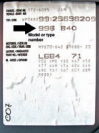
Model or type number location, which is the same for all 911 models from model year 1982.
