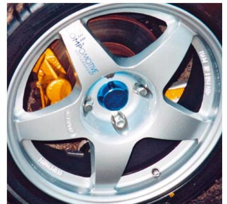
10-6 The brake caliper clearance offered by these superb Compomotive wheels is exemplary. The rims are 7in and are running 205 x 50 x 16in tyres, while also showing off the brake calipers (in this case SD1 Vitesse).
