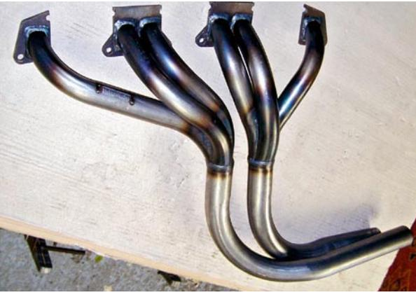
**3-4 The MGC exhaust manifold/header. It is preferable but not mandatory to fit a twin-pipe/twin-box exhaust system at the first opportunity ... although, to be fair, you will not lose much power and will be hard pushed to detect the difference if you retain your standard single-pipe/box system, at least until it comes time to replace the exhaust system.**
