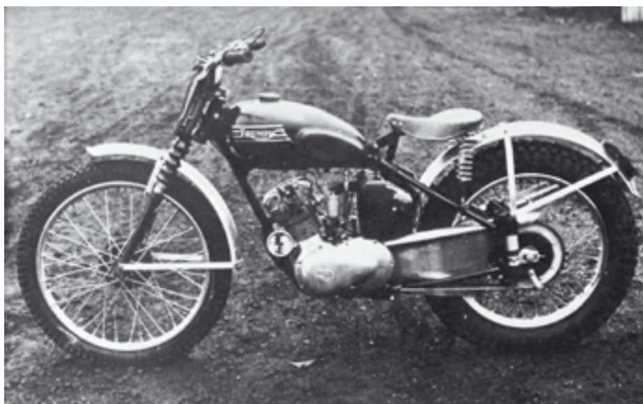
The trials version of the Terrier, built by Jim Alves in the workshop adjoining his motorcycle business in Glastonbury, Somerset. He modified a second-hand model bought in from a customer in a part-exchange deal. Meriden was not associated with this project in any way and had no intention of making a similar model.
