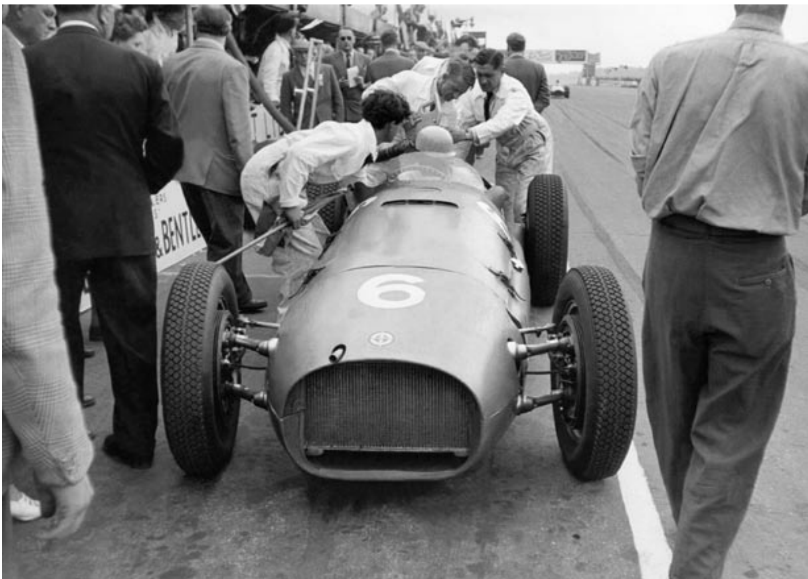
Fuel flowed into Reg Parnell's tank at a pit stop from BRM's Norton-powered pressure-delivery system. Vapour locks in the vent pipes from the scuttle tanks meant that both cars had to stop a second time for additional fuel.
