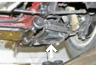
The front spring pans can rust through and, in severe cases, the front suspension could collapse.
