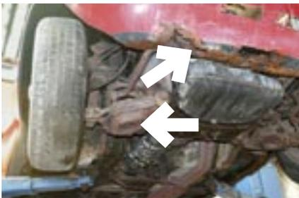
The crossmember beneath the radiator and the valance in front of it can both rot away, as can the front spring pans (both arrowed).
