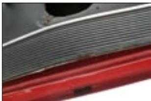
**Look to see that the drain holes beneath the doors are clear. Clear out with the blade of a screwdriver, if necessary.**
