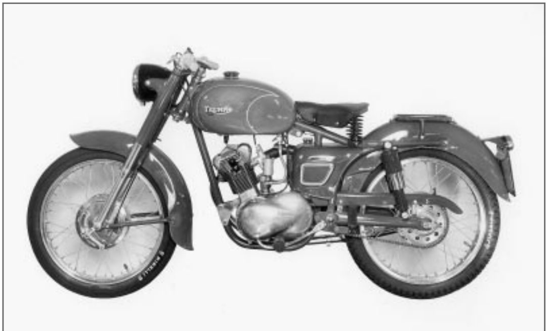
Fig. 3.20b The Fochj project - from the drive side. Note that it says 'Terrier' on the primary cover but '200cc' on the tank. (The Mike Estall Photo Collection)
