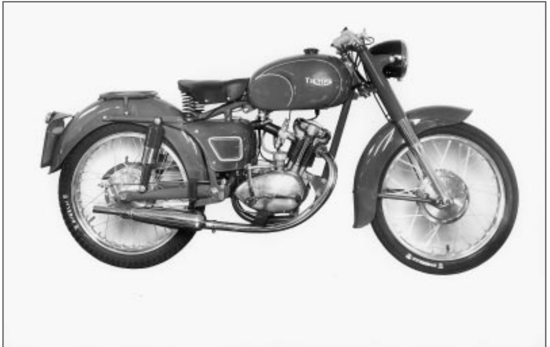
Fig. 3.20a An example of a Terrier-engined Fochj motor cycle - from the timing side. (The Mike Estall Photo Collection)
