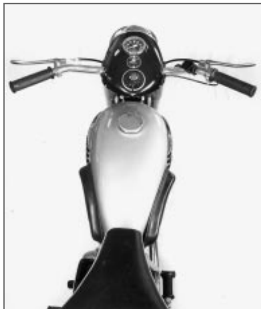
Fig 3.6a A late 1955 home market T20, viewed from above. Note the separate cable cut-outs in the nacelle - from no. 17258 onwards. (The Mike Estall Photo Collection)
