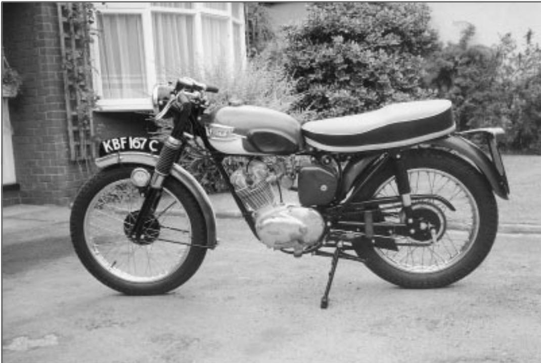
**Fig. 6.7b** The 1966 T20SH in Metallic Blue and Alaskan White, as it appeared in the sales brochure. In production the two colours followed the petrol tank seam and were not as illustrated here. (The Mike Estall Photo Collection)
