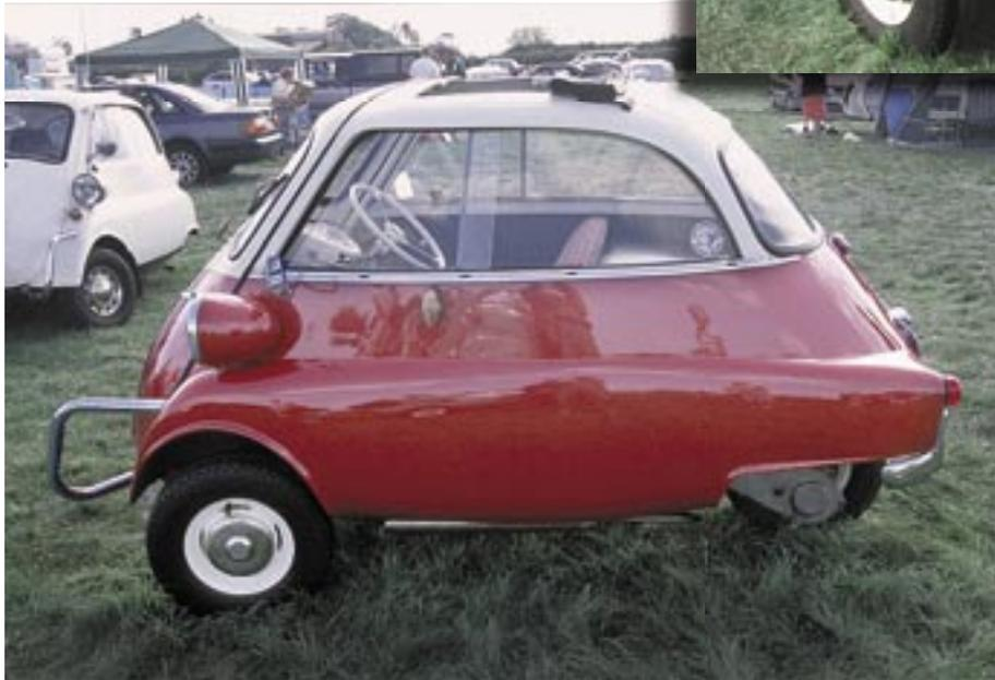
Pictured at an enthusiasts' rally this late model Isetta has right hand drive. The driver and the engine are positioned on the same side of the car which caused stability problems. So that the car would not overturn on right hand bends and corners, Isetta engineers devised a method of installing ballast. When unsuspecting owners removed the metal weight from the left hand side of the car, difficulties in maintaining equilibrium were encountered.
