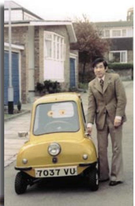
Above: Another bubble-oddy is the Peel, the most diminutive car built in the United Kingdom. The prototype machine featured a single wheel at the front but following testing the configuration was reversed. When the Peel P50 first appeared in 1962 the bubblecar era was virtually over, but priced at a little under £200 it nevertheless attracted some customers. Around 50 P50s were made, each fitted with a 49cc DKW fan-cooled two-stroke which afforded a breathtaking 40mph. (Gordon Fitzgerald)
