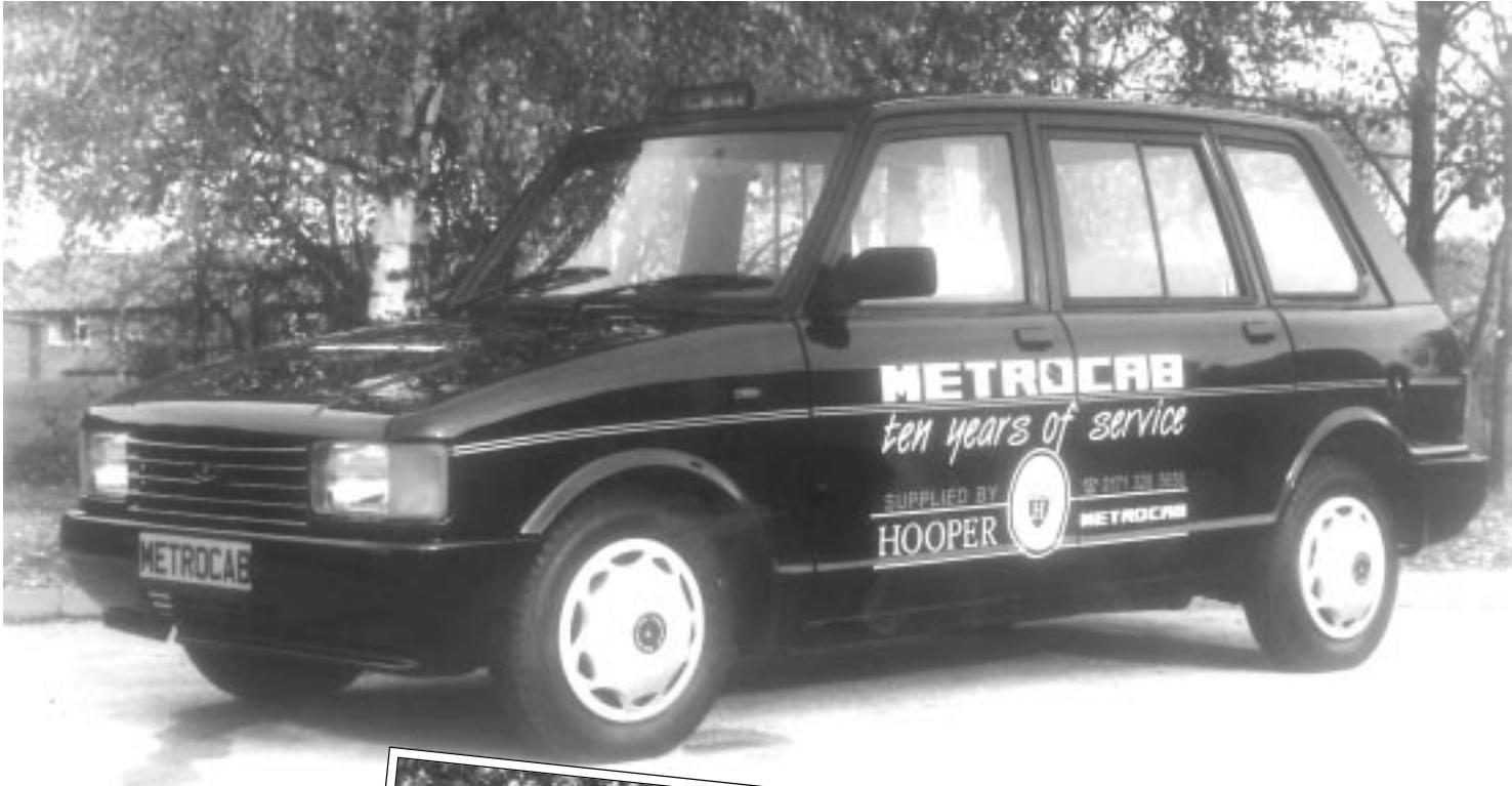
Above: Many owner-drivers elect to buy the Metrocab which, like the Fairway, is designed to fully comply with Scotland Yard regulations. The glass reinforced plastic (GRP) body is impervious to corrosion and styling is more modern than the Fairway. In areas of the UK, such as Scotland, where corrosion is a problem, the Metrocab is especially popular. (Courtesy Hooper Metrocab and Stratford Marketing)
