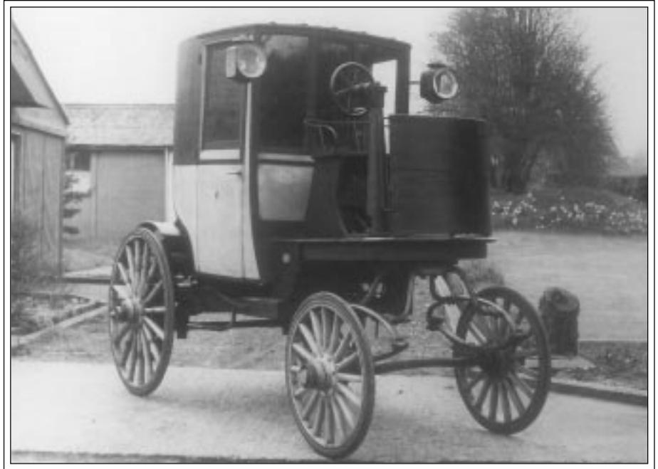
The first motorised taxicab to operate in London was the electrically propelled Bersey, named after its designer, C. W. Bersey. Entering service with the London Electric Cab Company during August 1897, the Berseys were soon nicknamed "Humming Birds" because of the sound of their motors. The cabs had a 30 mile (48km) range between charging periods and a maximum speed of 9mph (14.5kph).
