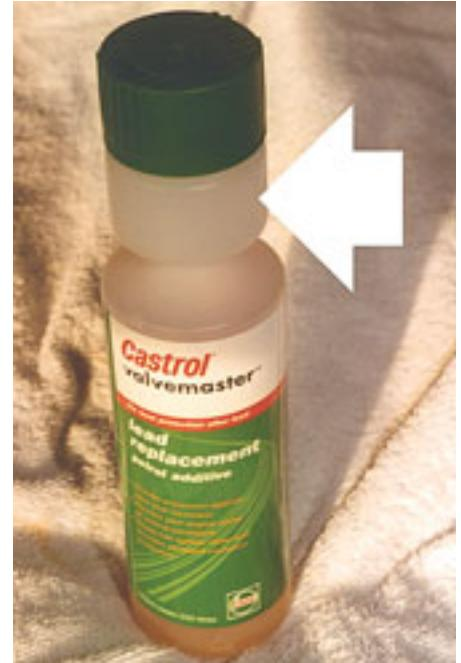
**6-10-1** An example of AWAs (Anti-wear additives) intended to reduce valve seat recession (VSR). The bottle is squeezed until the top measuring part (arrowed) is filled.
