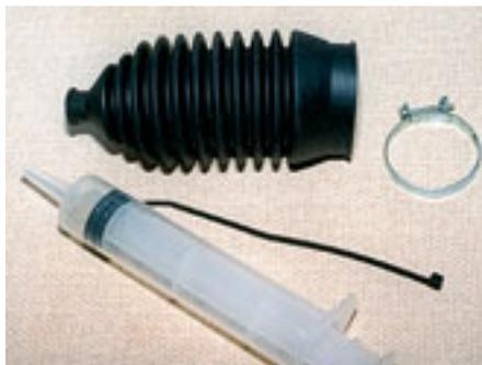
**10-11-1 (Picture 7) ...**a syringe will be necessary to inject the (thickish) EP90 oil into the rack through the small end of the gaiter. You may or may not get a cable tie-type clip in your kit...
