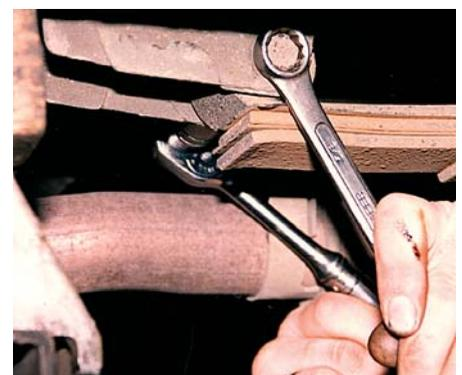
12-8-1 (Picture 10) ...Finally, tighten the eye bolt with the car's weight on the axle.
