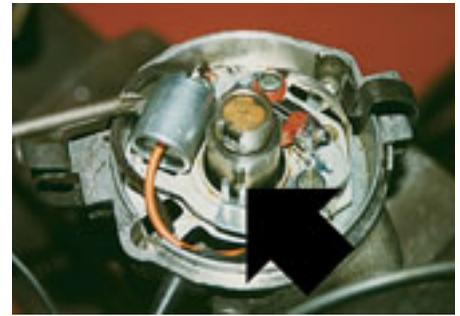
**3-1-4 (Picture 1) This picture shows the condenser (screwdriver points to it), the distributor cam (arrowed) and gives another general view of the Lucas 45D distributor...**
