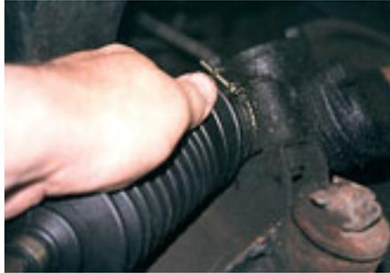
**10-11-1 (Picture 6)** Once the inner end of the gaiter is secured to the rack with the clip supplied in most gaiter kits...
