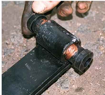
12-8-1 (Picture 7) Use lots of copper-based grease at every stage of reassembly, and remember that the springs are heavy; get help to offer up each replacement.
