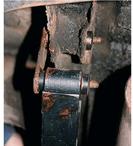
12-8-1 (Picture 8) You may need to compress the spring to lengthen it sufficiently to get the shackle into place (before fitting the plate)...
