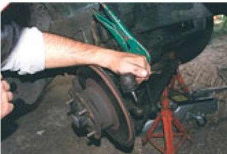
**10-11-1 (Picture 4) ...**separate the tapered shoulder on the ball joint from the track control arm.
