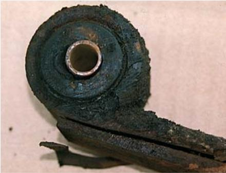
12-8-1 (Picture 3) It looks as if this central tube has separated from its bonded rubber bush, and certainly needs replacing. Since the spring also looks well used, this is clearly a case for a new pair of rear springs.
