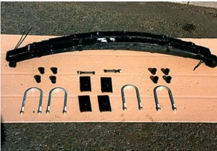
12-8-1 (Picture 4) Order a complete kit, as shown here. Safely support both car and axle, and change one spring at a time.
