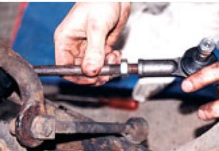
**10-11-1 (Picture 5)** Count the number of turns off the trackrod for each ball joint, and the number back on again, although it's still best to get the tracking checked afterward.
