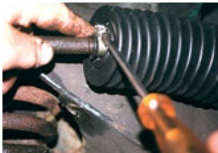
**10-11-1 (Picture 8) ...**but one will be necessary to seal the small end of the gaiter to the trackrod.
