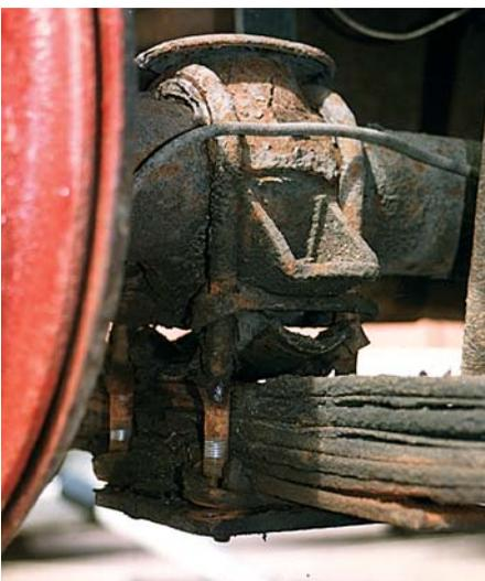
12-8-1 (Picture 5) In addition to the front eye fastening, remove the two U-bolts...
