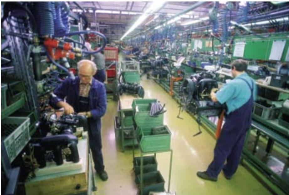
*The 993 was built in a far more efficient manner than its predecessors. These pictures show engines being put together, and front suspension units for the rear-wheel drive Carreras on the production lines in the background.*
